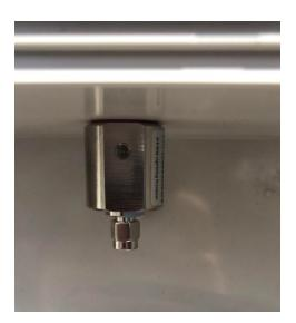
7. Thread the male end of the bluetooth cable into the female end of the lightning arrester and fasten the female end of the cable to male end of the RTU (outlined in light blue)
