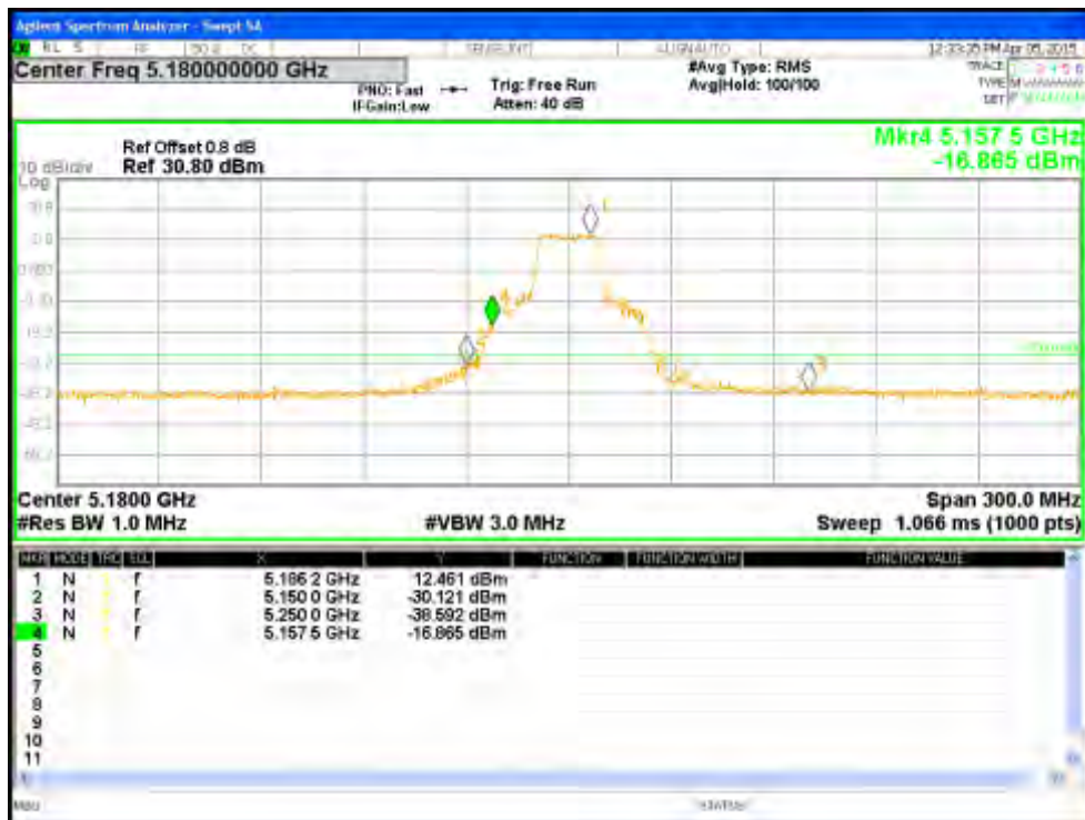
Figure 113: Measured Bandedge for VHT20-Nss1 MCS0 at 5180 MHz, Chain 0
