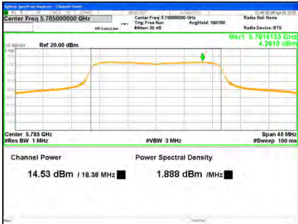
Figure 16: Maximum Transmitted Power, 5785 MHz at VHT20 Nss2 MCS0, Chain 0
