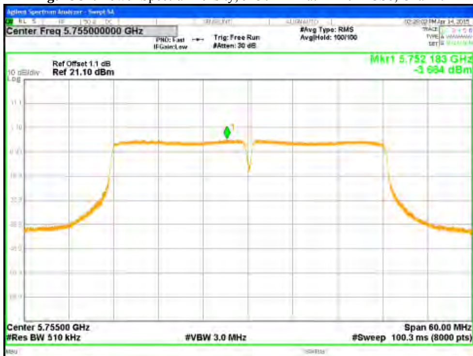
Figure 92: Power Spectral Density, 5755 MHz at HT40 MCS8, Chain 0
