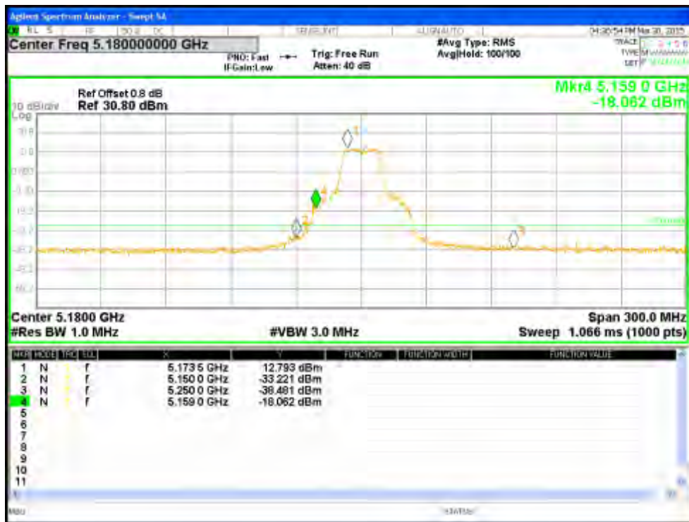
Figure 101: Measured Bandedge for 802.11a-6Mbps at 5180 MHz, Chain 0
