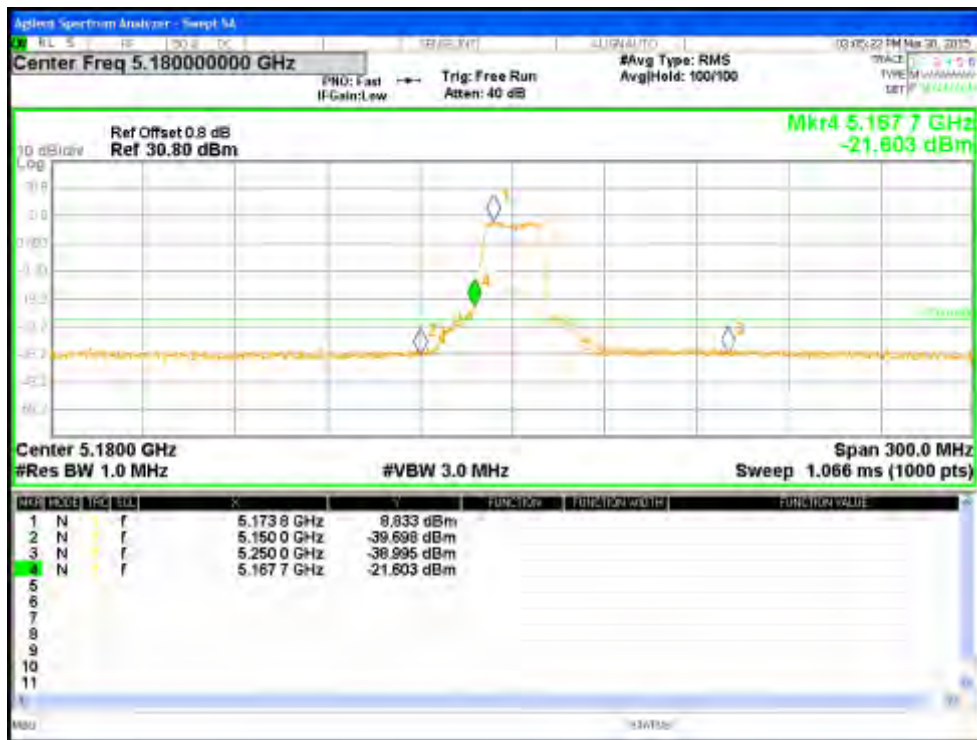
Figure 111: Measured Bandedge for HT20-MCS8 at 5180 MHz, Chain 1
