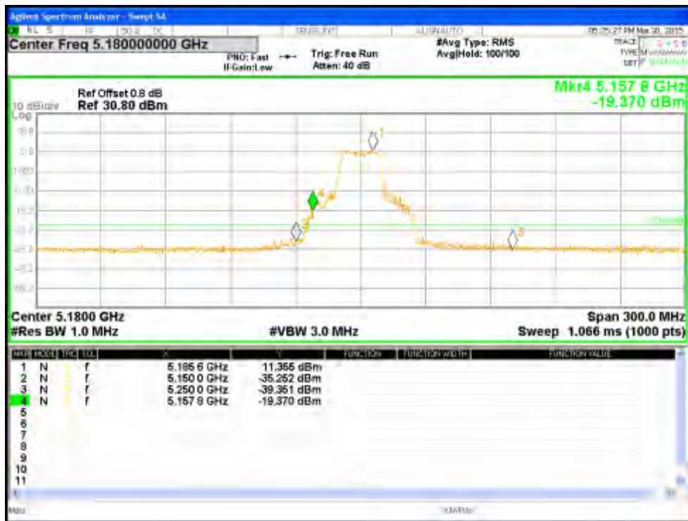
Figure 107: Measured Bandedge for HT20-MCS0 at 5180 MHz, Chain 1
