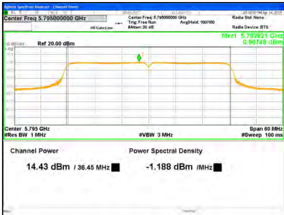
Figure 25: Maximum Transmitted Power, 5795 MHz at VHT40 Nss1 MCS0, Chain 0
