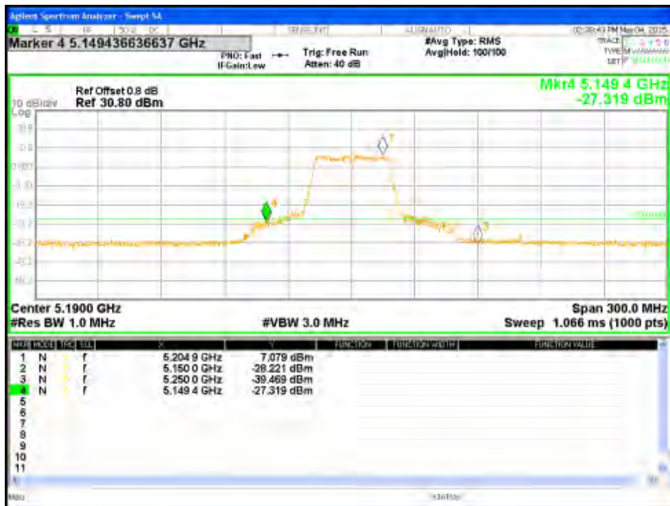
Figure 133: Measured Bandedge for VHT40-Nss2 MCS0 at 5190 MHz, Chain 0
