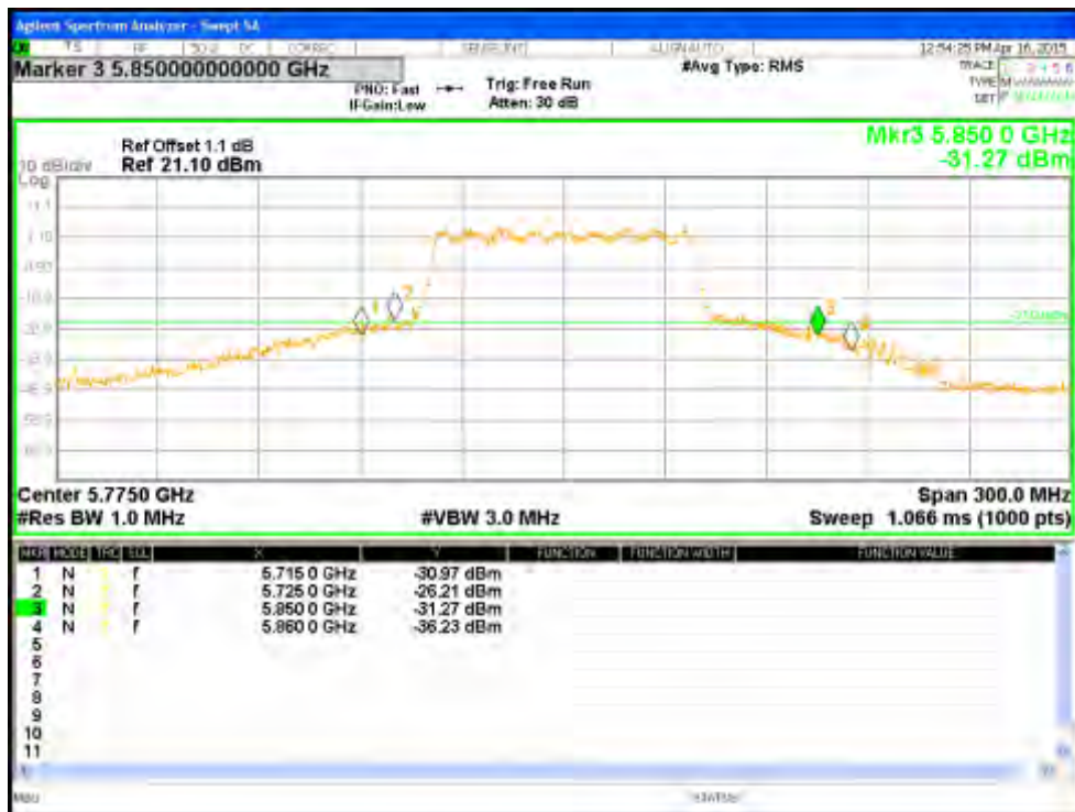
Figure 181: Measured Bandedge for VHT80-Nss1 MCS0 at 5775 MHz, Chain 0
