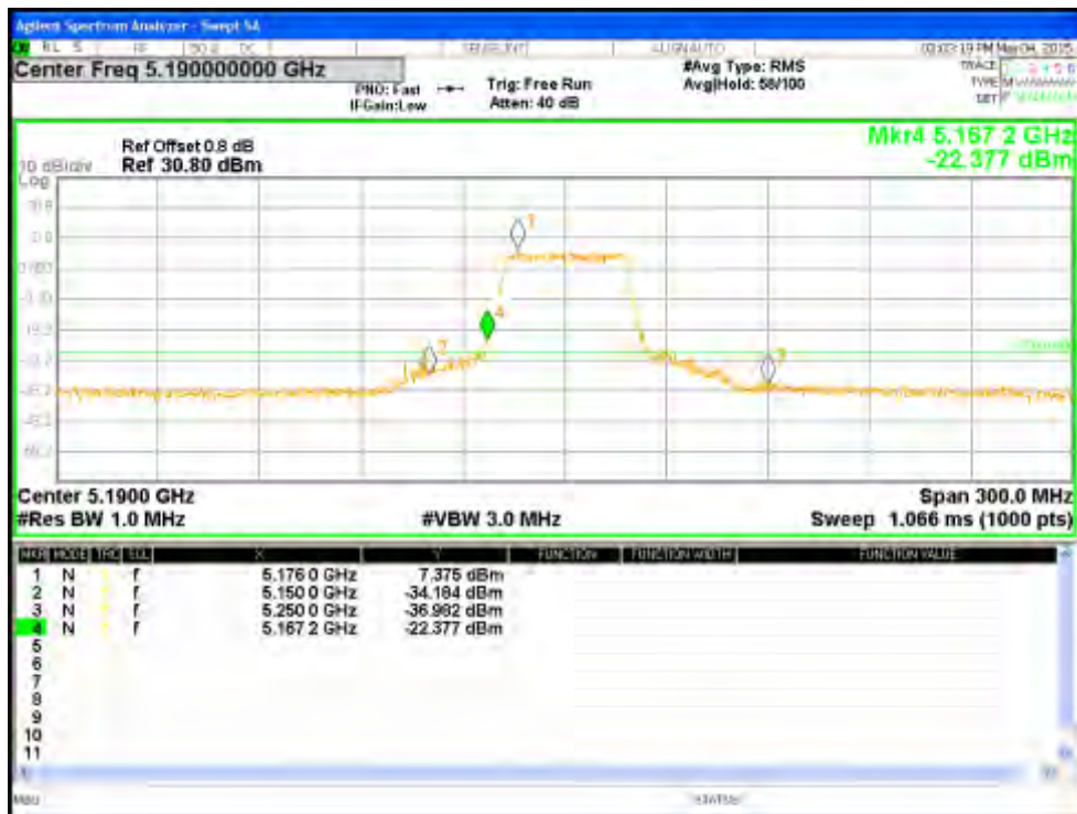
Figure 135: Measured Bandedge for VHT40-Nss2 MCS0 at 5190 MHz, Chain 1
