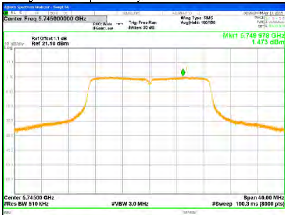
Figure 82: Power Spectral Density, 5745 MHz at HT20 MCS0, Chain 0
