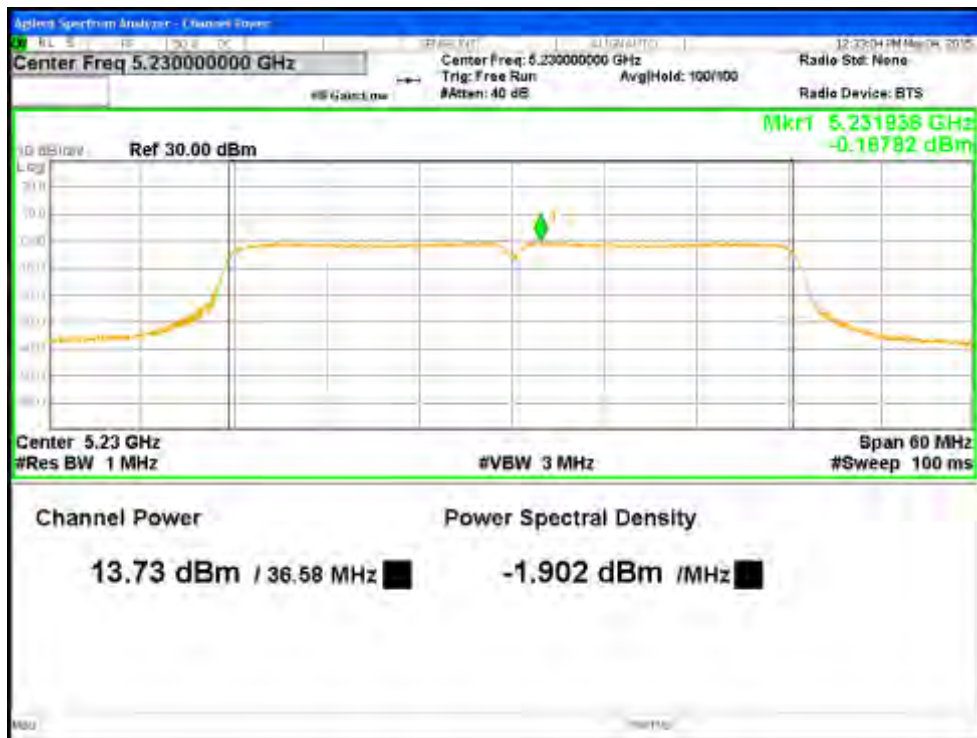
Figure 21: Maximum Transmitted Power, 5230 MHz at HT40 MCS8, Chain 0
