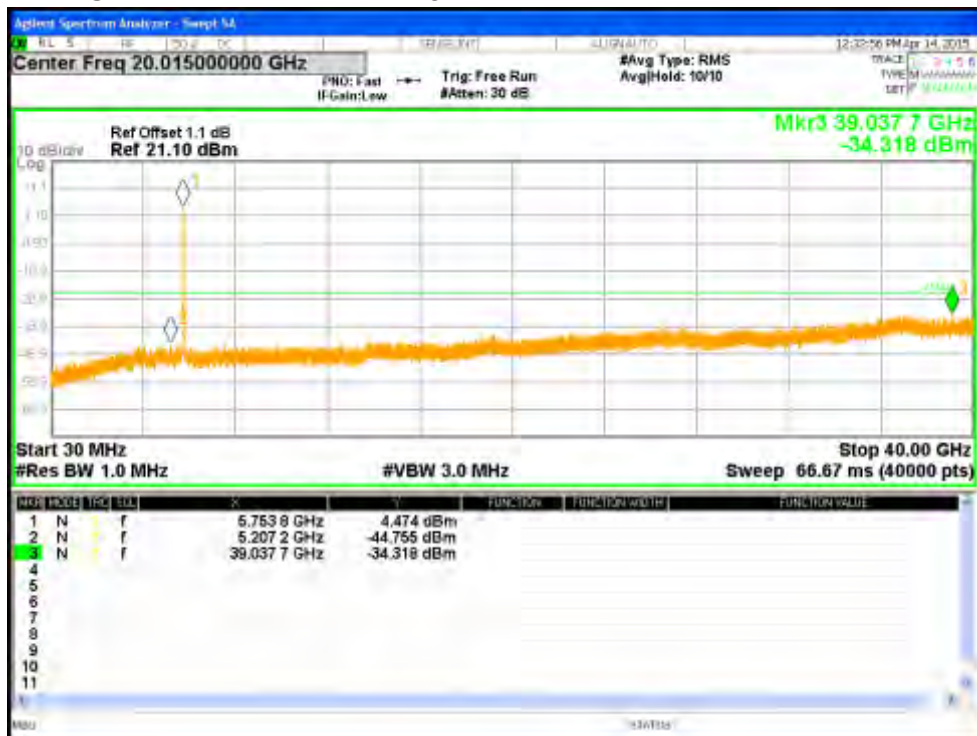
Figure 168: Undesirable Emission for HT40-MCS0 at 5755 MHz, Chain 1
