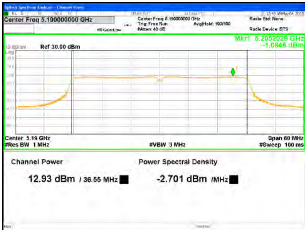
Figure 18: Maximum Transmitted Power, 5190 MHz at HT40 MCS0, Chain 1
