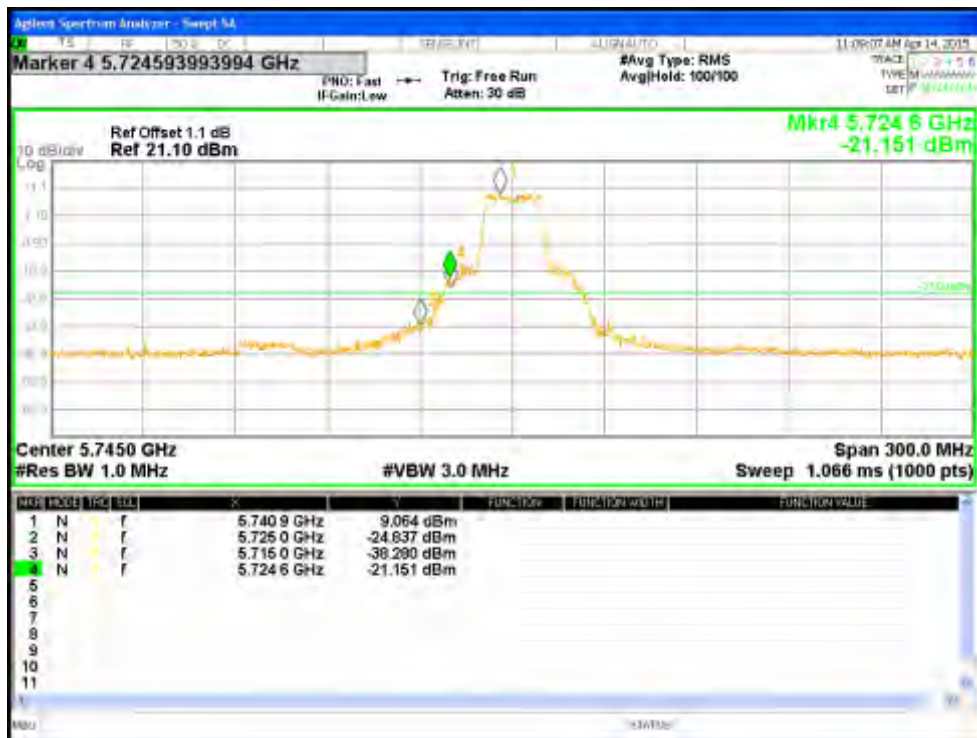
Figure 155: Measured Bandedge for HT20-MCS8 at 5745 MHz, Chain 1
