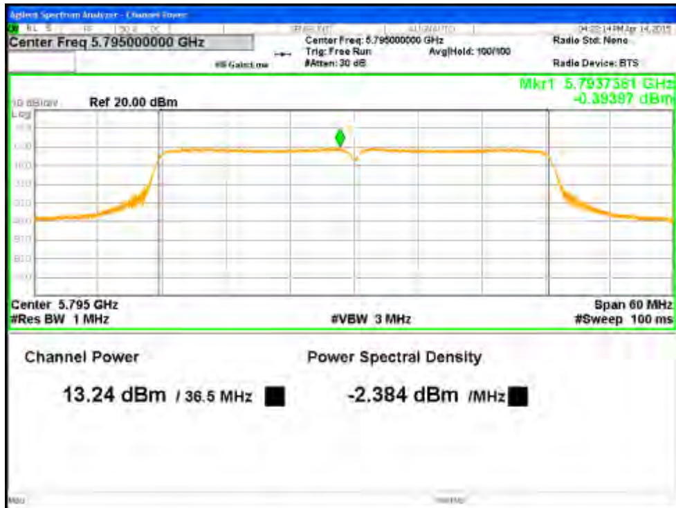
Figure 28: Maximum Transmitted Power, 5795 MHz at VHT40 Nss2 MCS0, Chain 0
