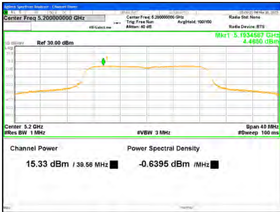
Figure 9: Maximum Transmitted Power, 5200 MHz at HT20 MCS8, Chain 0
