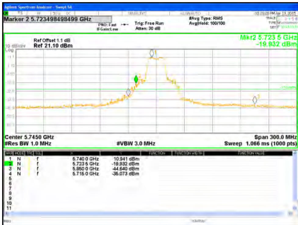
Figure 149: Measured Bandedge for HT20-MCS0 at 5745 MHz, Chain 0
