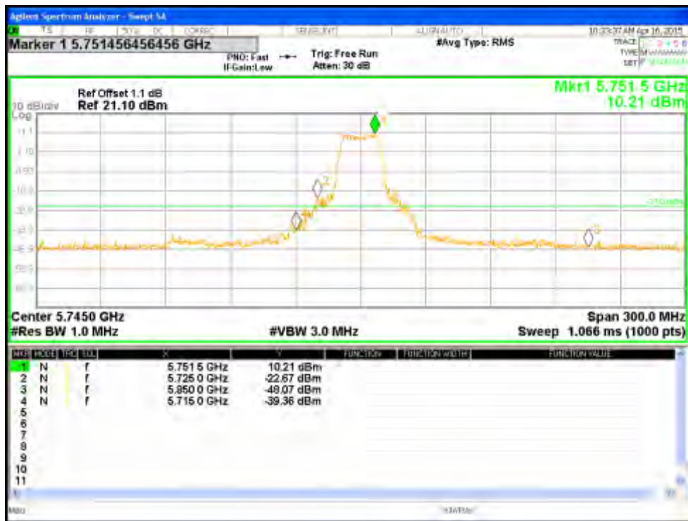
Figure 159: Measured Bandedge for VHT20-Nss1 MCS0 at 5745 MHz, Chain 1
