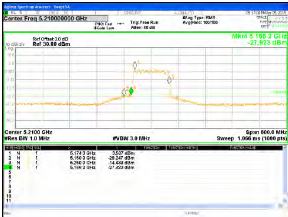
Figure 141: Measured Bandedge for VHT80-Nss2 MCS0 at 5190 MHz, Chain 0
