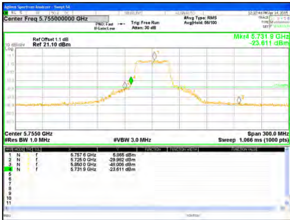
Figure 167: Measured Bandedge for HT40-MCS0 at 5755 MHz, Chain 1
