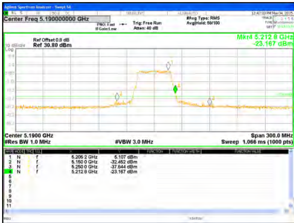
Figure 127: Measured Bandedge for HT40-MCS8 at 5190 MHz, Chain 1
