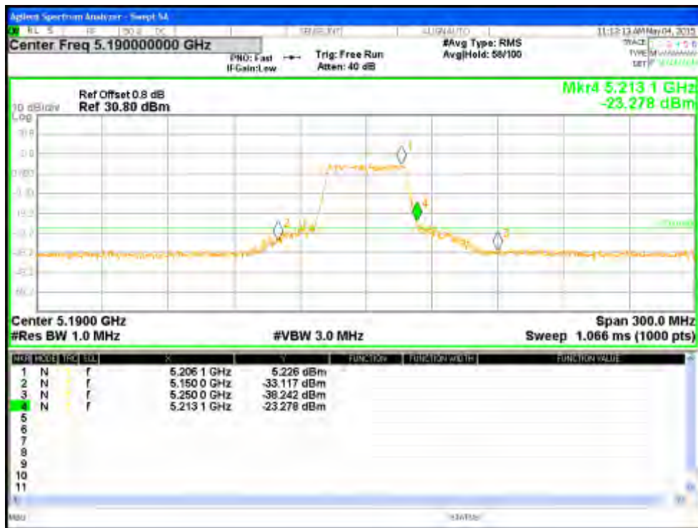
Figure 123: Measured Bandedge for HT40-MCS0 at 5190 MHz, Chain 1
