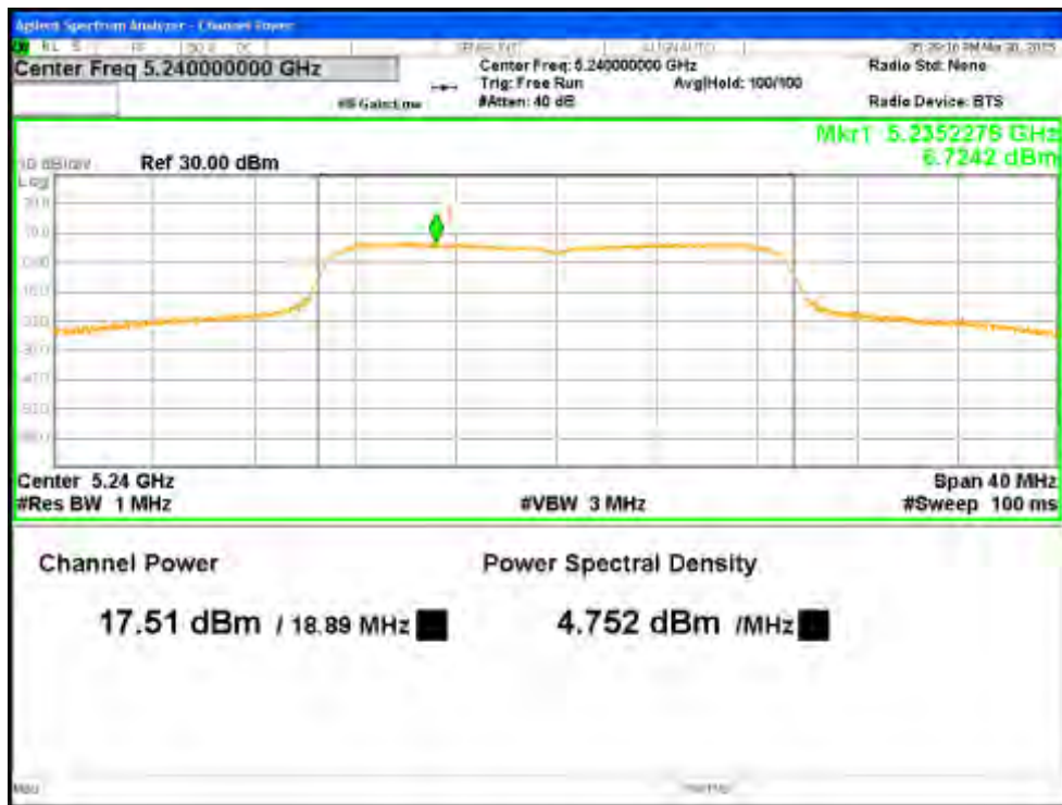
Figure 5: Maximum Transmitted Power, 5240 MHz at HT20 MCS0, Chain 0
