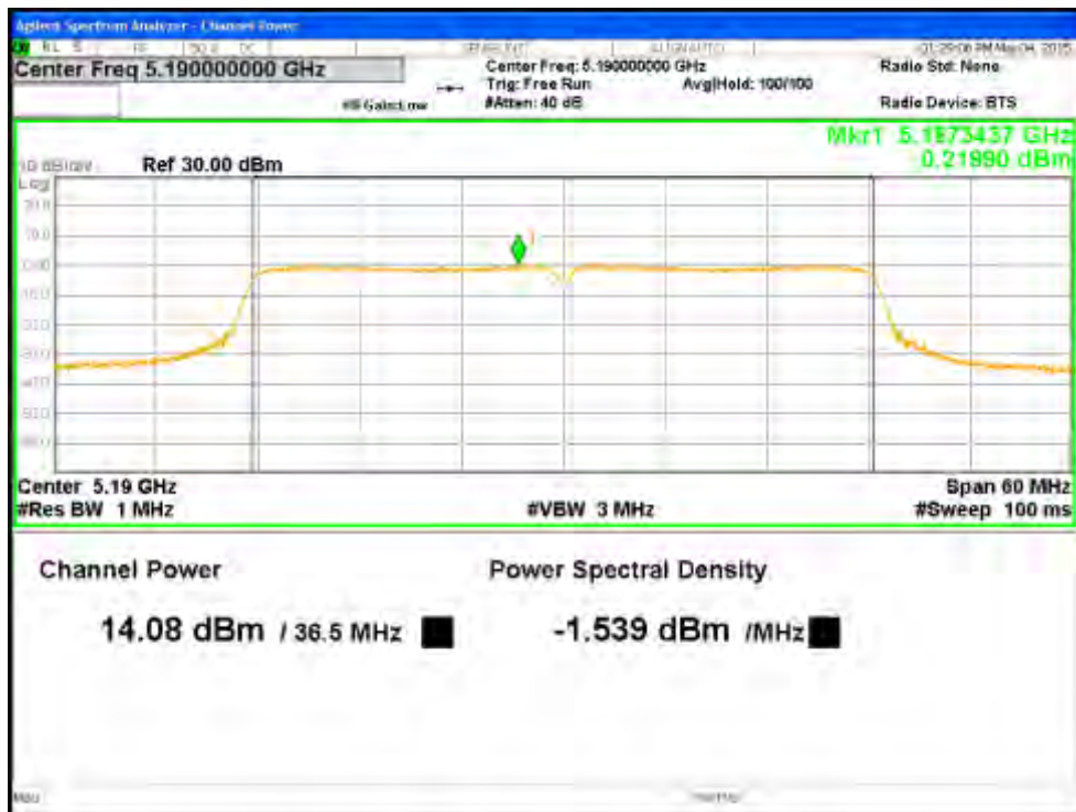
Figure 23: Maximum Transmitted Power, 5190 MHz at VHT40 Nss1 MCS0, Chain 0
