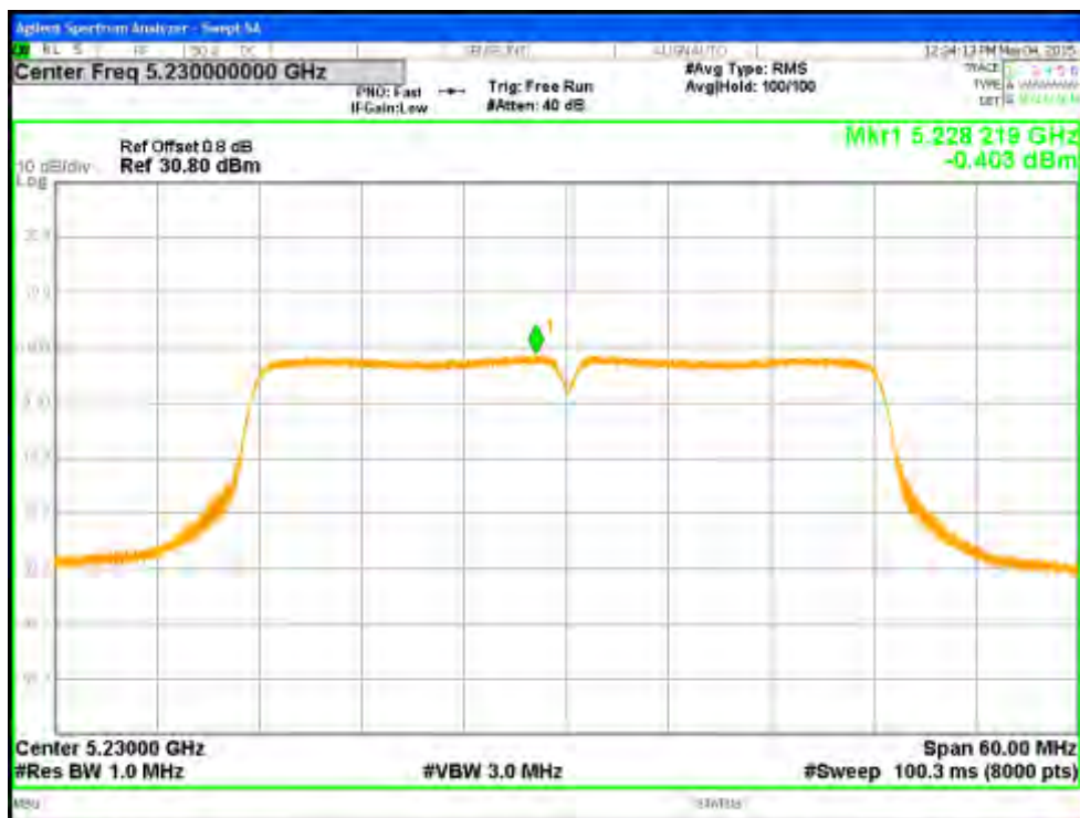
Figure 91: Power Spectral Density, 5230 MHz at HT40 MCS8, Chain 0
