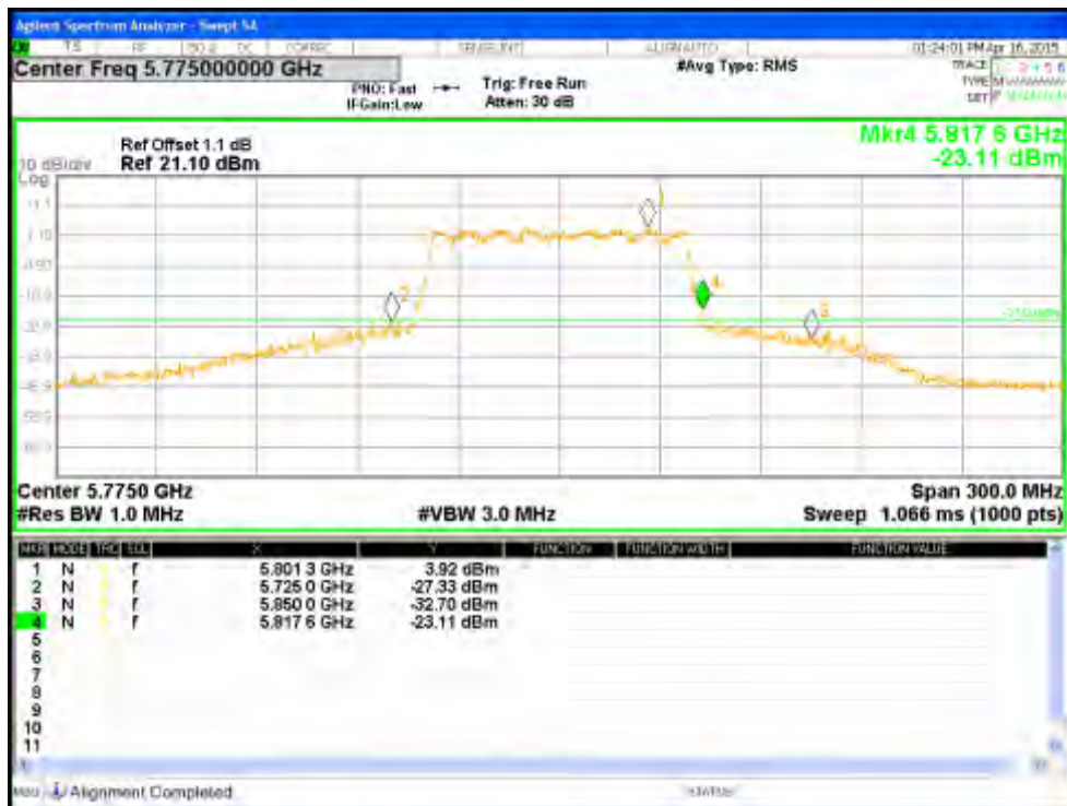
Figure 185: Measured Bandedge for VHT80-Nss2 MCS0 at 5775 MHz, Chain 0
