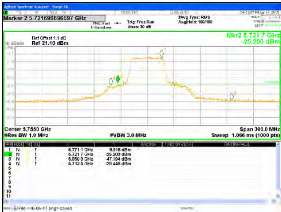
Figure 177: Measured Bandedge for VHT40-Nss2 MCS0 at 5755 MHz, Chain 0
