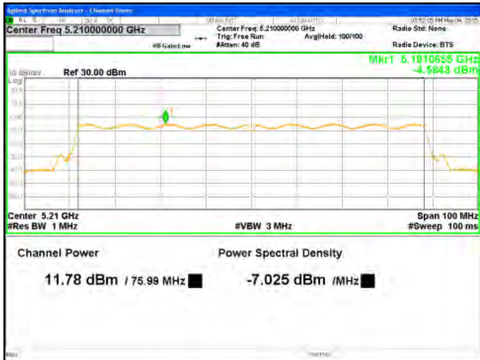
Figure 30: Maximum Transmitted Power, 5210 MHz at VHT80 Nss1 MCS0, Chain 1
