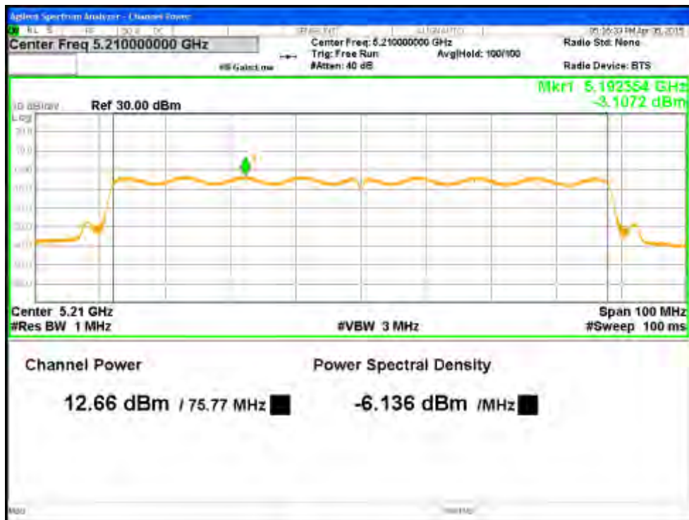
Figure 33: Maximum Transmitted Power, 5210 MHz at VHT80 Nss2 MCS0, Chain 0
