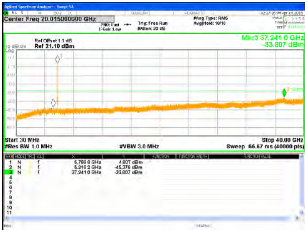
Figure 170: Undesirable Emission for HT40-MCS8 at 5755 MHz, Chain 0
