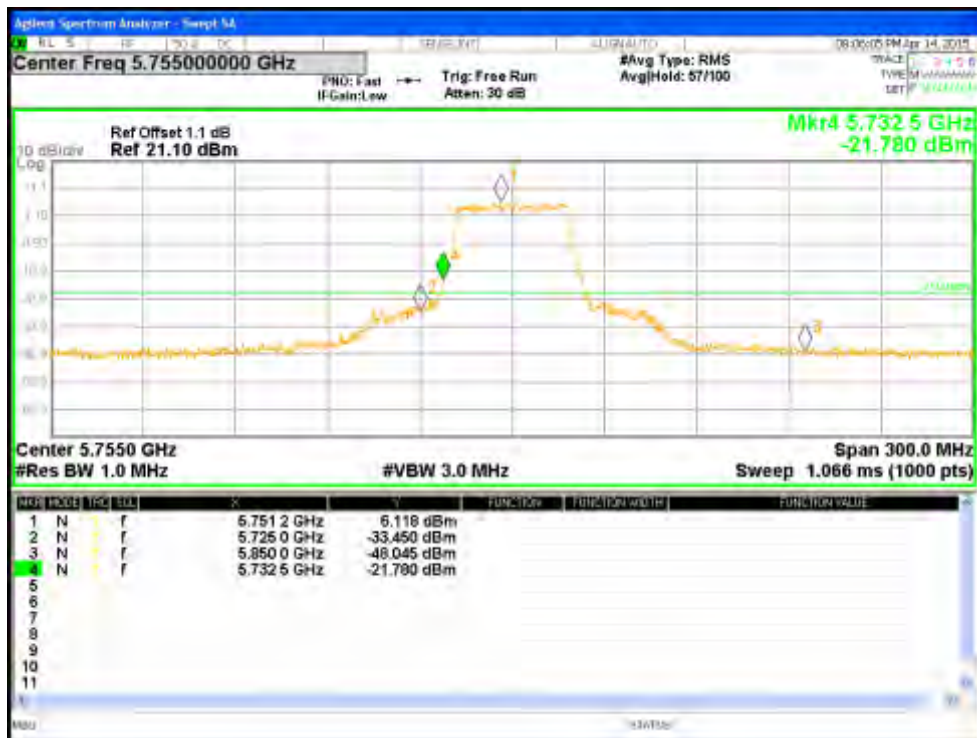
Figure 179: Measured Bandedge for VHT40-Nss2 MCS0 at 5755 MHz, Chain 1
