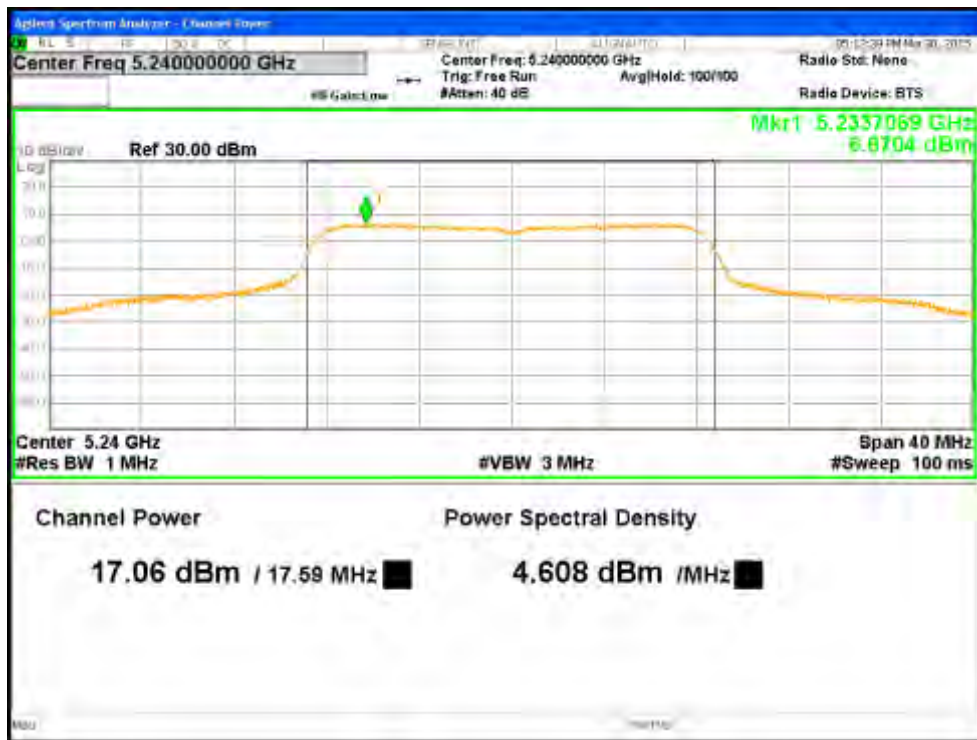
Figure 1: Maximum Transmitted Power, 5240 MHz at 11a, Chain 0
