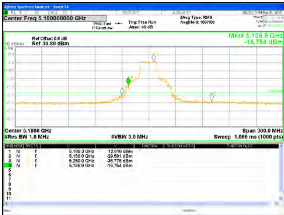
Figure 105: Measured Bandedge for HT20-MCS0 at 5180 MHz, Chain 0
