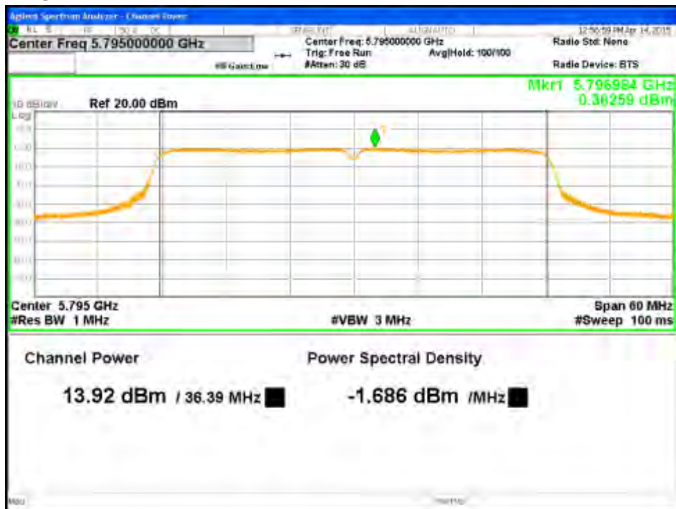
Figure 20: Maximum Transmitted Power, 5795 MHz at HT40 MCS0, Chain 1
