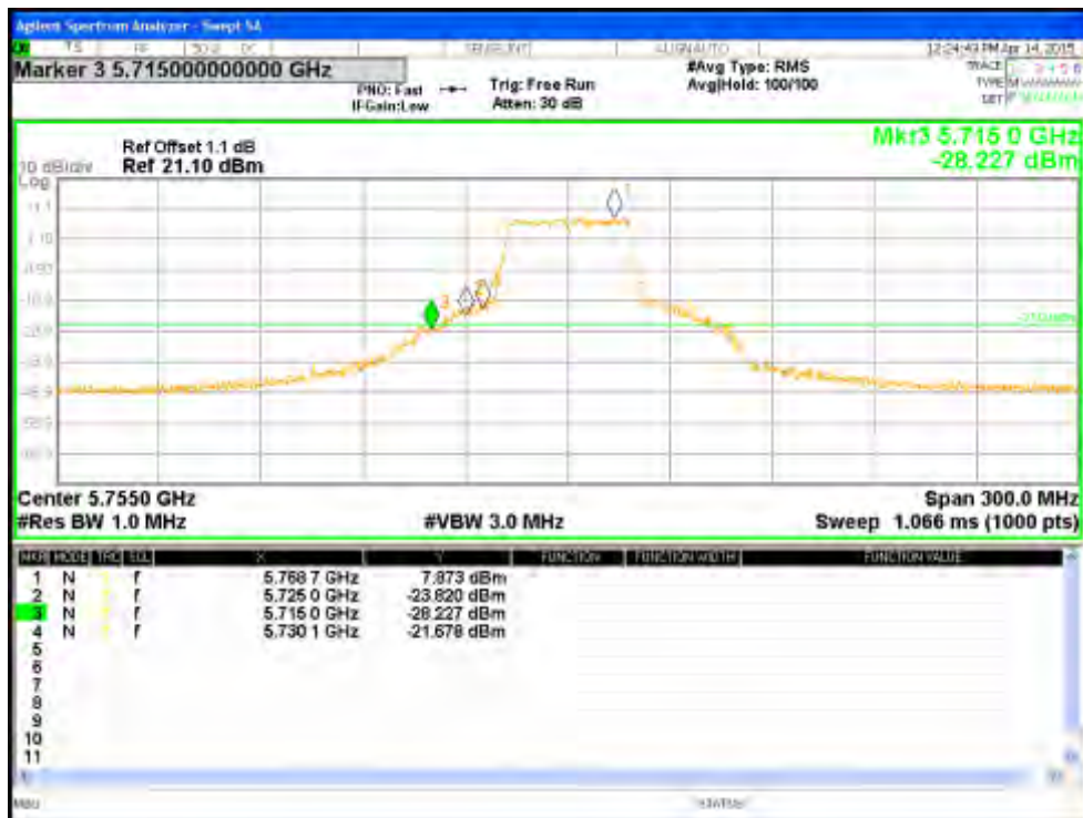
Figure 165: Measured Bandedge for HT40-MCS0 at 5755 MHz, Chain 0
