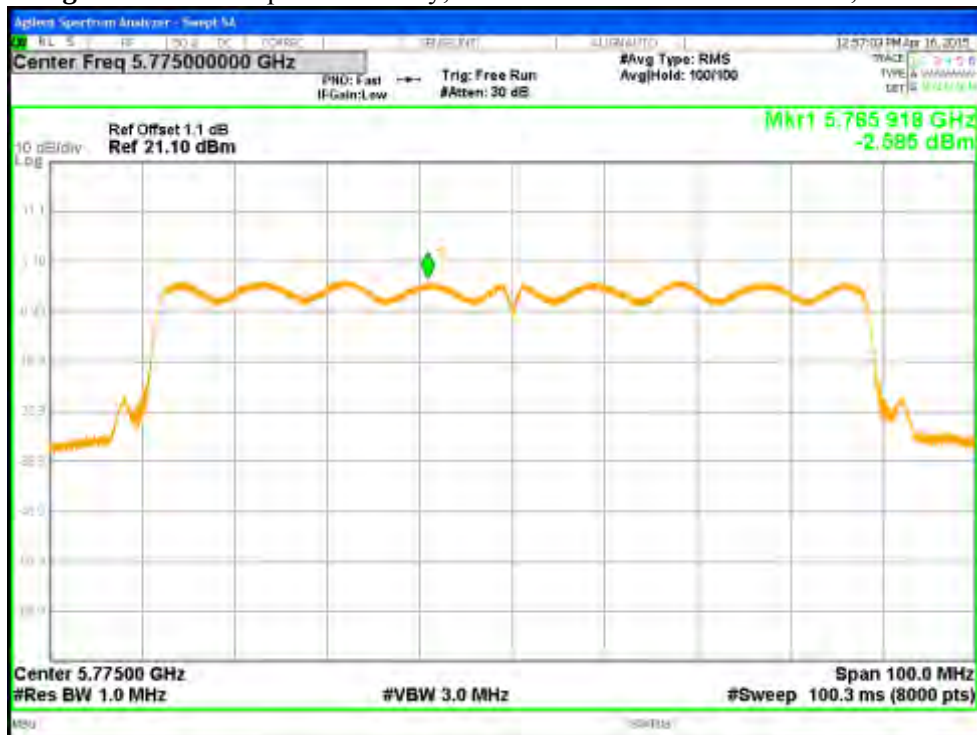
Figure 98: Power Spectral Density, 5775 MHz at VHT80 Nss1 MCS0, Chain 0
