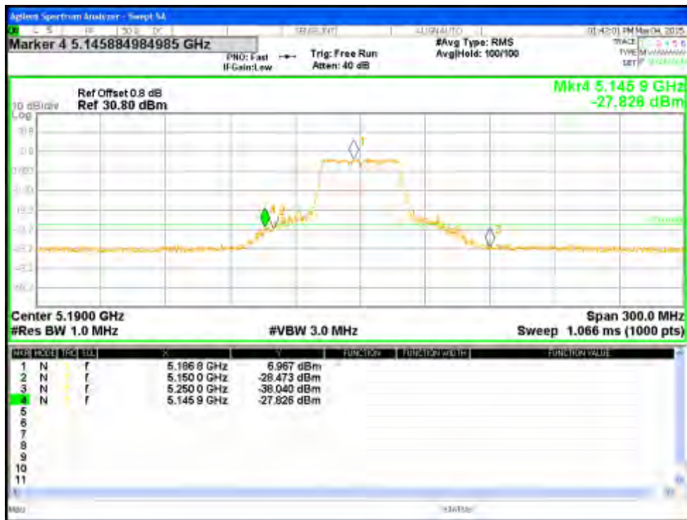
Figure 129: Measured Bandedge for VHT40-Nss1 MCS0 at 5190 MHz, Chain 0
