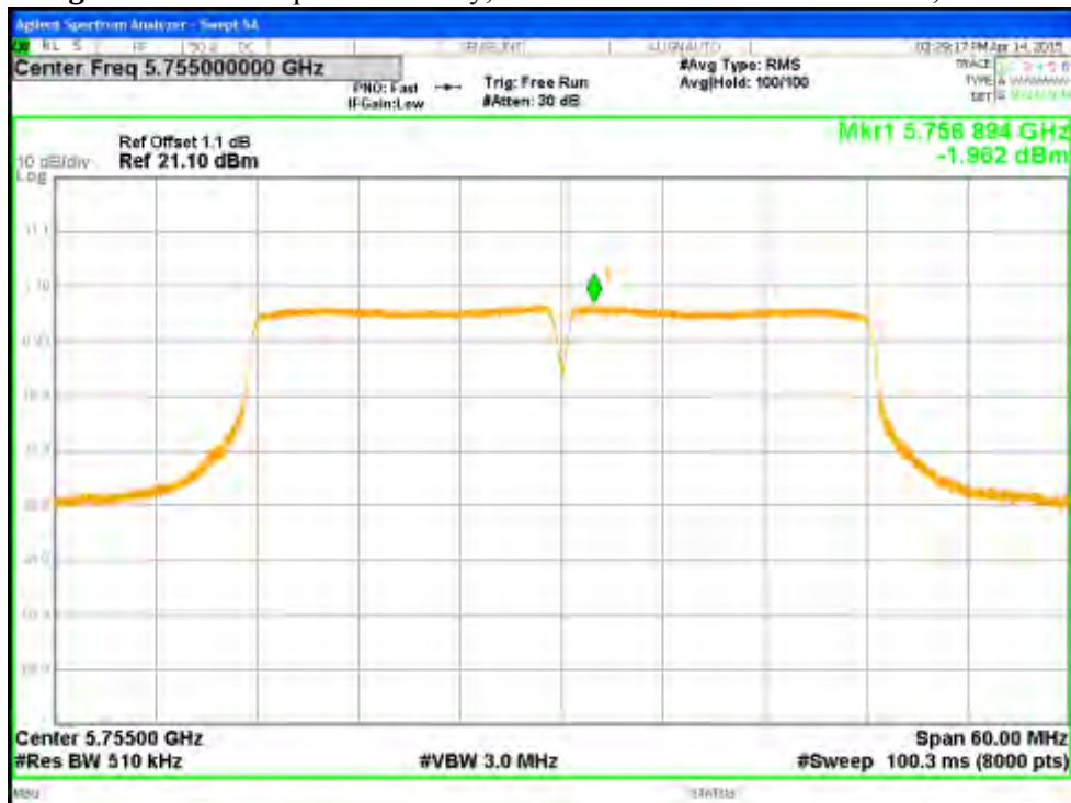
Figure 94: Power Spectral Density, 5755 MHz at VHT40 Nss1 MCS0, Chain 0
