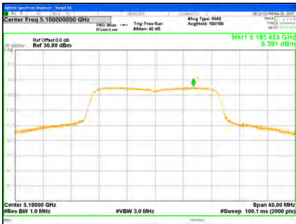
Figure 81: Power Spectral Density, 5180 MHz at HT20 MCS0, Chain 0
