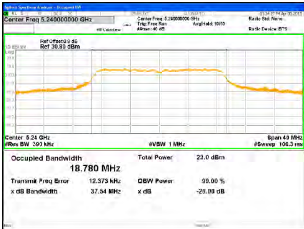
Figure 48: 26dB & 99% Occupied Bandwidth, 5240 MHz at VHT20 Nss1 MCS0, Chain 1
