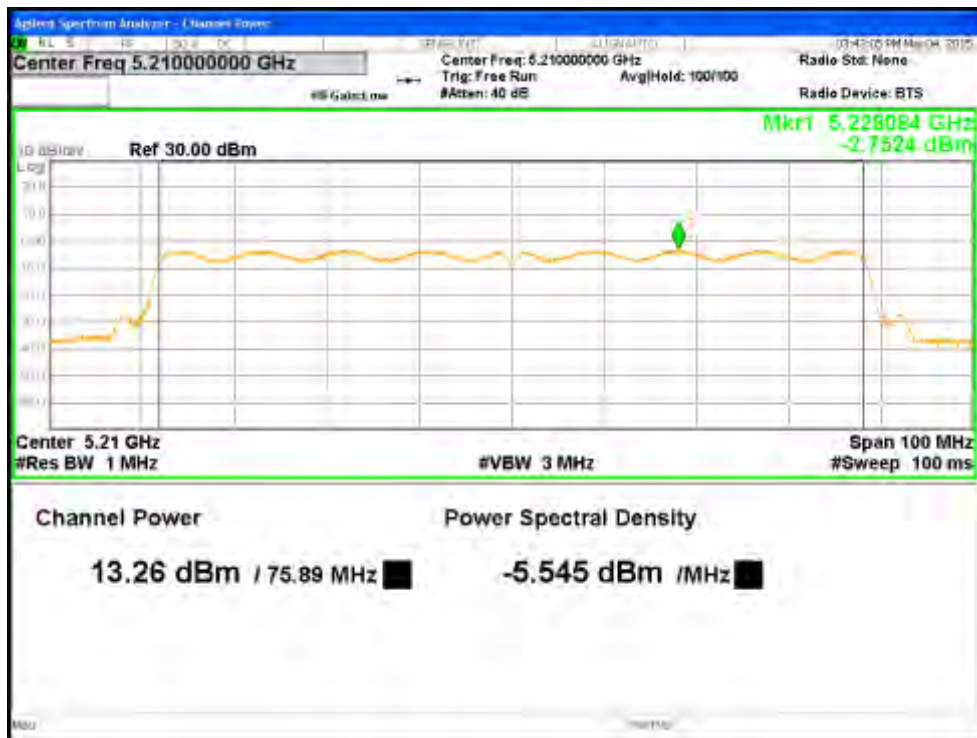
Figure 29: Maximum Transmitted Power, 5210 MHz at VHT80 Nss1 MCS0, Chain 0
