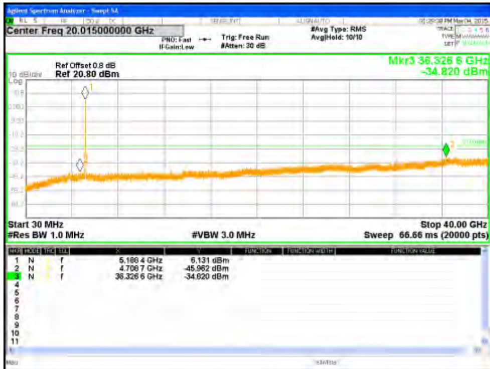
Figure 130: Undesirable Emission for VHT40-Nss1 MCS0 at 5190 MHz, Chain 0
