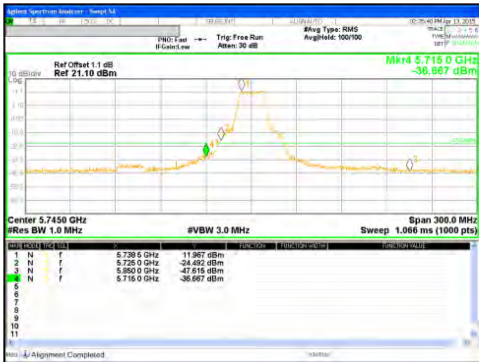
Figure 147: Measured Bandedge for 802.11a-6Mbps at 5745 MHz, Chain 1
