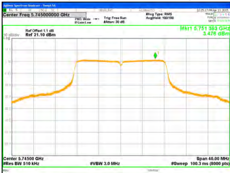
Figure 80: Power Spectral Density, 5745 MHz at 802.11a 6Mbps, Chain 0
