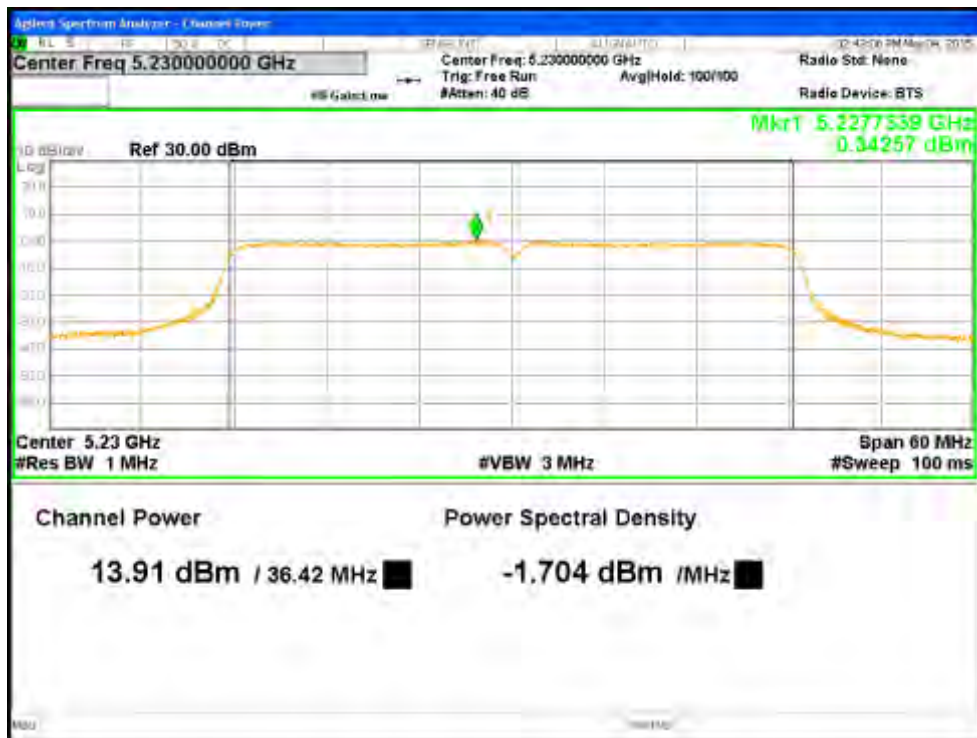
Figure 27: Maximum Transmitted Power, 5230 MHz at VHT40 Nss2 MCS0, Chain 0
