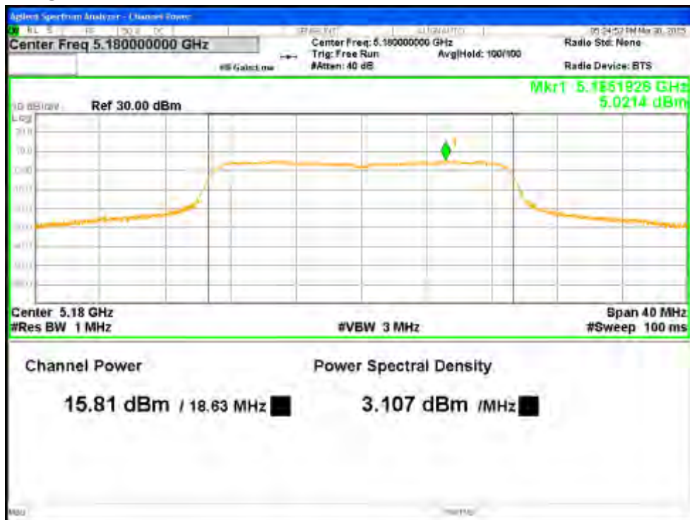
Figure 6: Maximum Transmitted Power, 5180 MHz at HT20 MCS0, Chain 1
