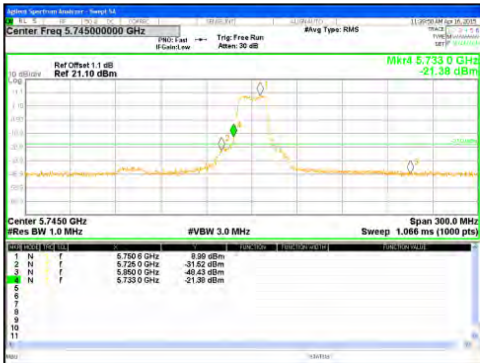
Figure 163: Measured Bandedge for VHT20-Nss2 MCS0 at 5745 MHz, Chain 1
