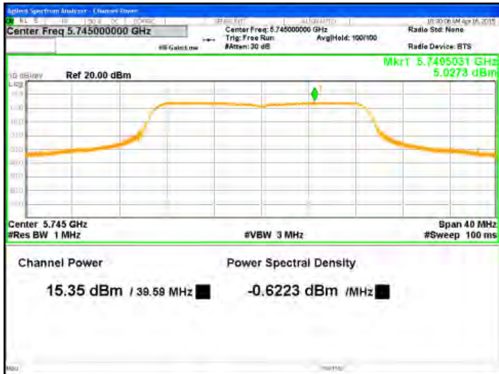
Figure 14: Maximum Transmitted Power, 5745 MHz at VHT20 Nss1 MCS0, Chain 1
