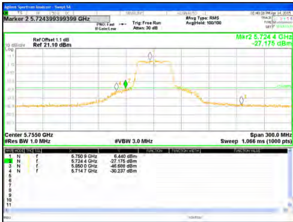
Figure 169: Measured Bandedge for HT40-MCS8 at 5755 MHz, Chain 0
