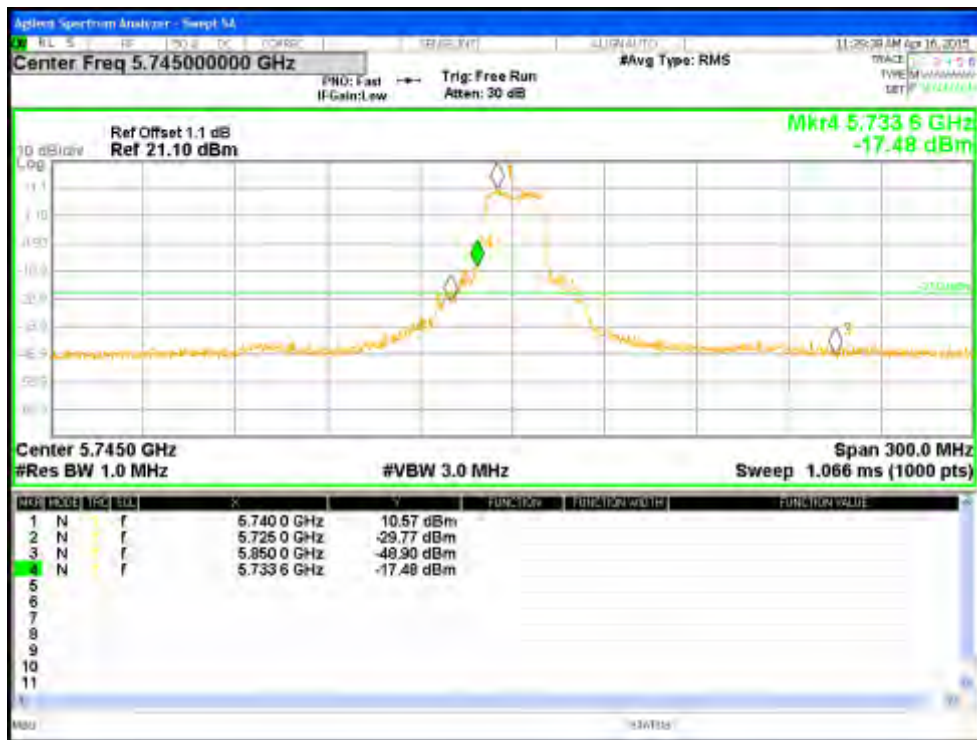
Figure 161: Measured Bandedge for VHT20-Nss2 MCS0 at 5745 MHz, Chain 0
