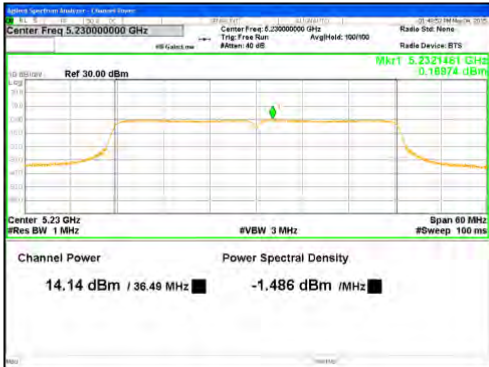
Figure 24: Maximum Transmitted Power, 5230 MHz at VHT40 Nss1 MCS0, Chain 0
