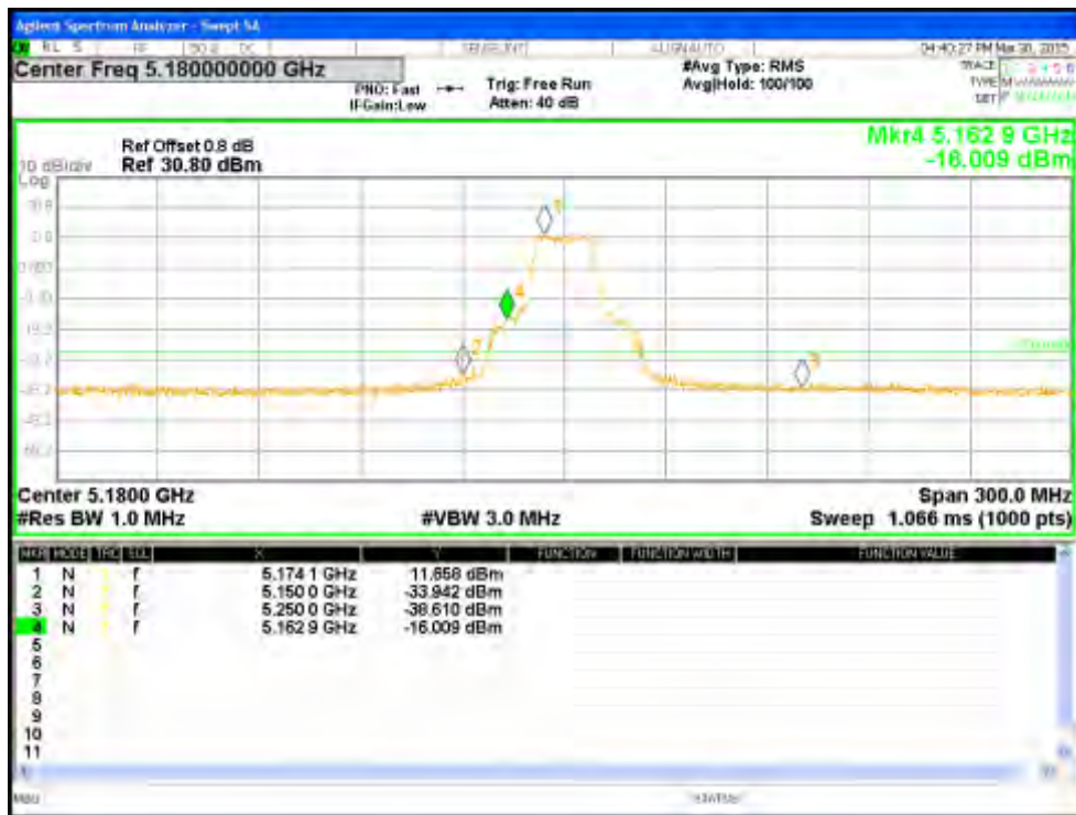
Figure 103: Measured Bandedge for 802.11a-6Mbps at 5180 MHz, Chain 1
