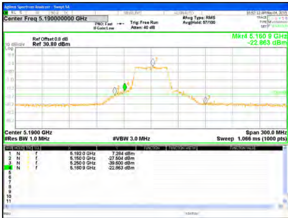
Figure 121: Measured Bandedge for HT40-MCS0 at 5190 MHz, Chain 0
