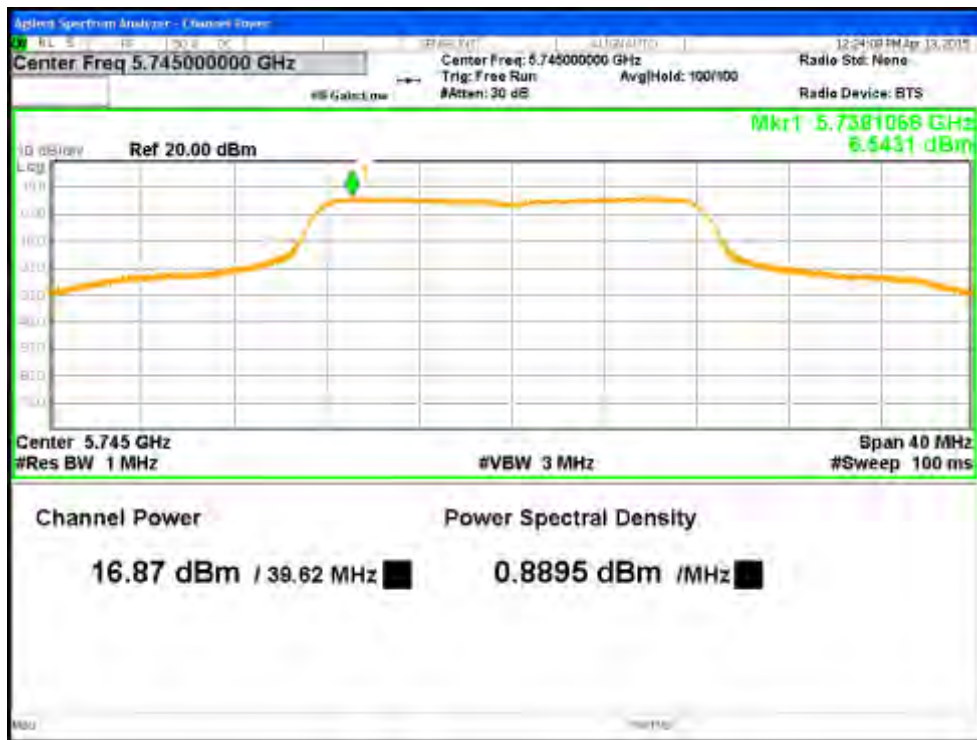
Figure 3: Maximum Transmitted Power, 5745 MHz at 11a, Chain 0
