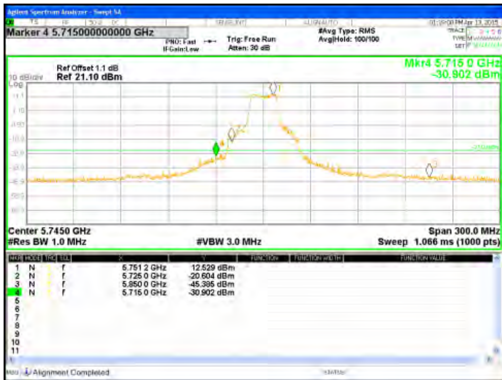
Figure 145: Measured Bandedge for 802.11a-6Mbps at 5745 MHz, Chain 0
