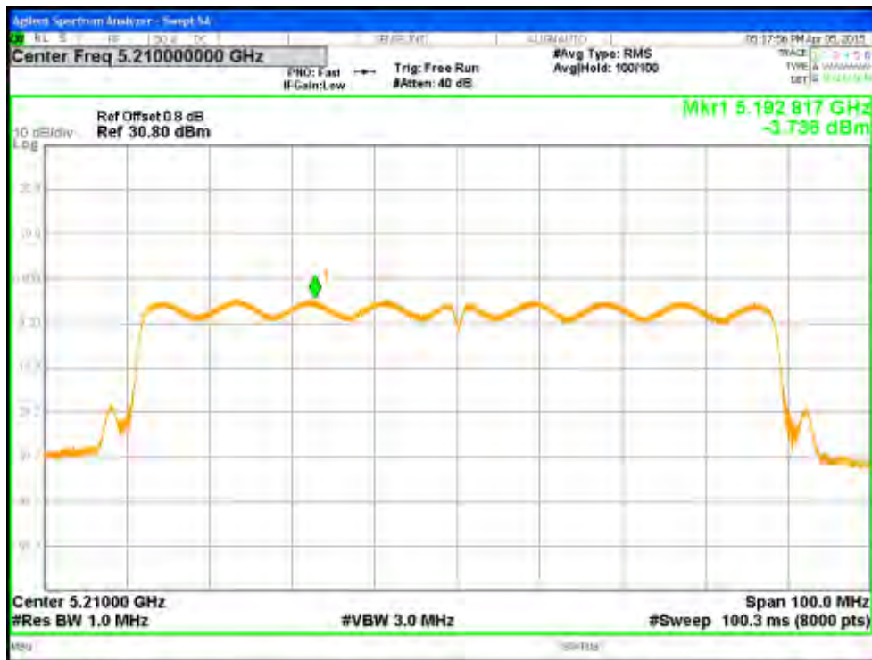
Figure 99: Power Spectral Density, 5210 MHz at VHT80 Nss2 MCS0, Chain 0
