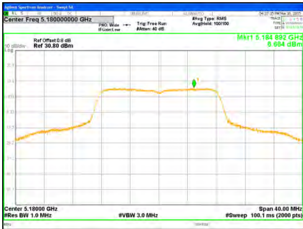
Figure 79: Power Spectral Density, 5180 MHz at 802.11a 6Mbps, Chain 0
