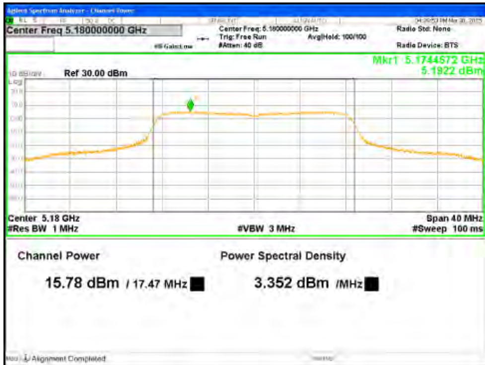
Figure 2: Maximum Transmitted Power, 5180 MHz at 11a, Chain 1
