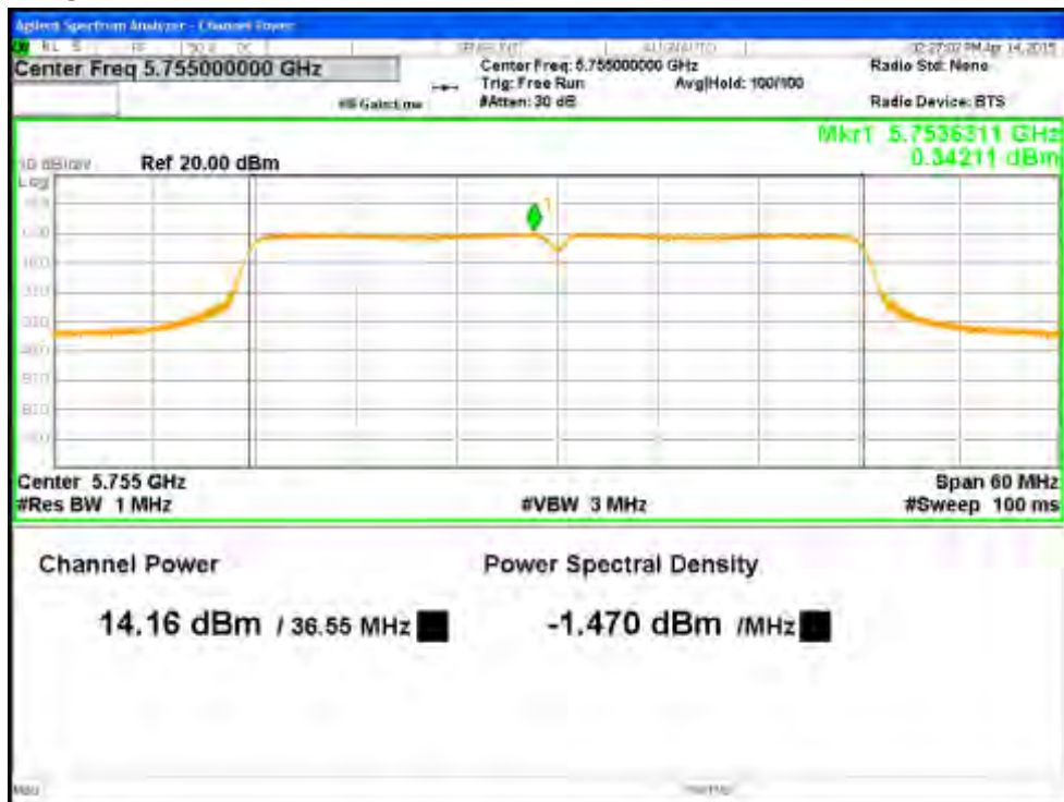
Figure 22: Maximum Transmitted Power, 5755 MHz at HT40 MCS8, Chain 0
