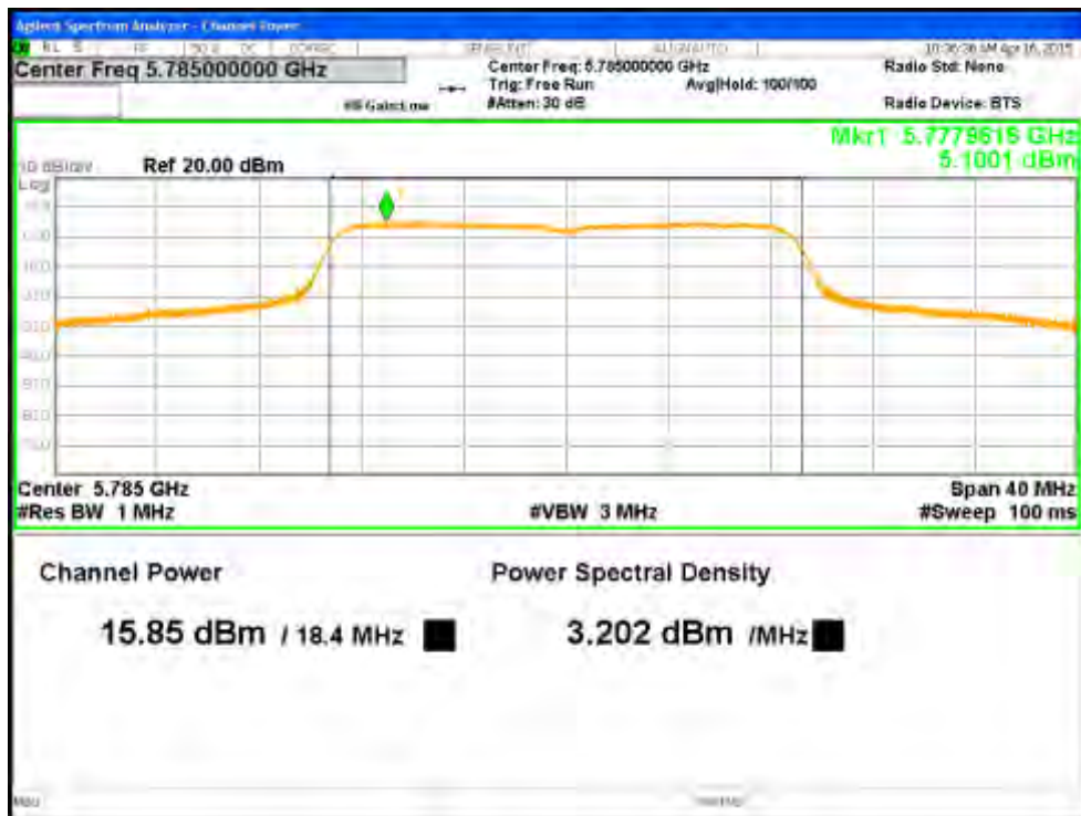
Figure 13: Maximum Transmitted Power, 5785 MHz at VHT20 Nss1 MCS0, Chain 0
