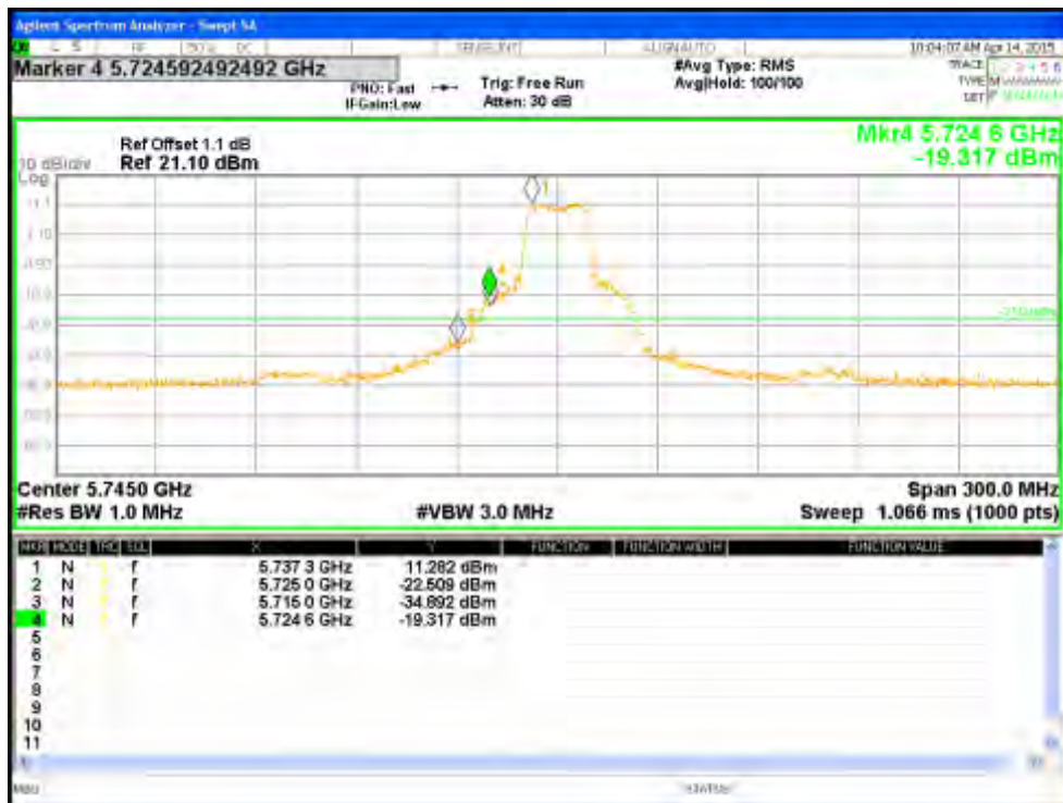
Figure 153: Measured Bandedge for HT20-MCS8 at 5745 MHz, Chain 0
