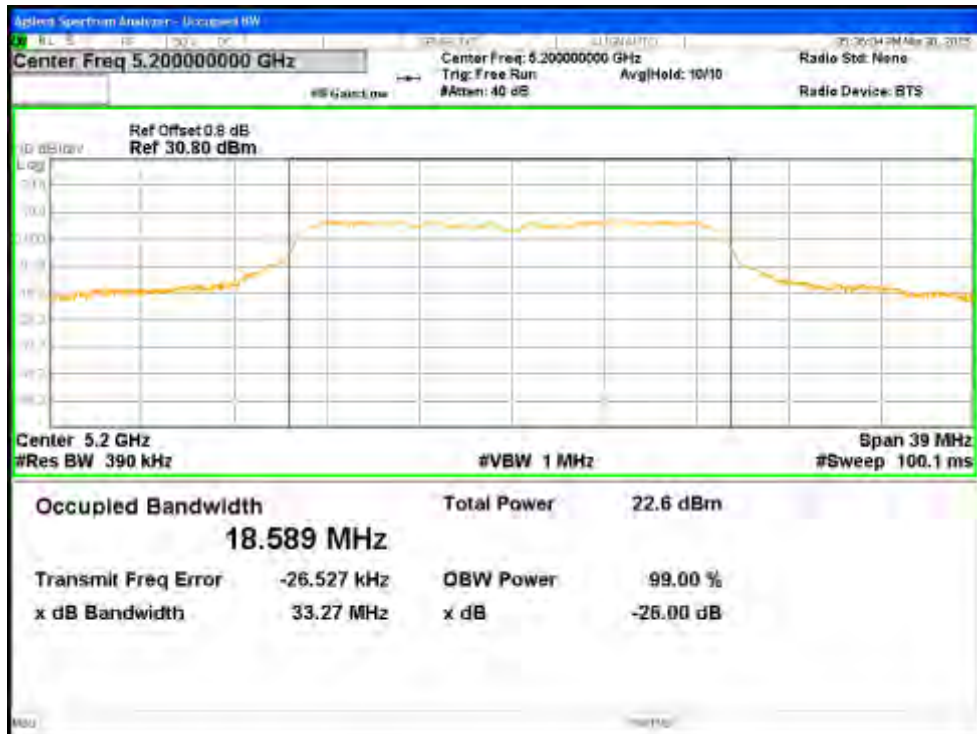
Figure 40: 26dB & 99% Occupied Bandwidth, 5200 MHz at HT20 MCS0, Chain 1
