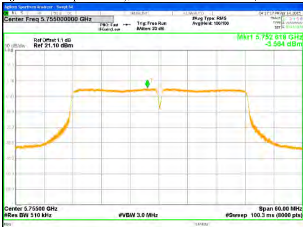
Figure 96: Power Spectral Density, 5755 MHz at VHT40 Nss2 MCS0, Chain 0
