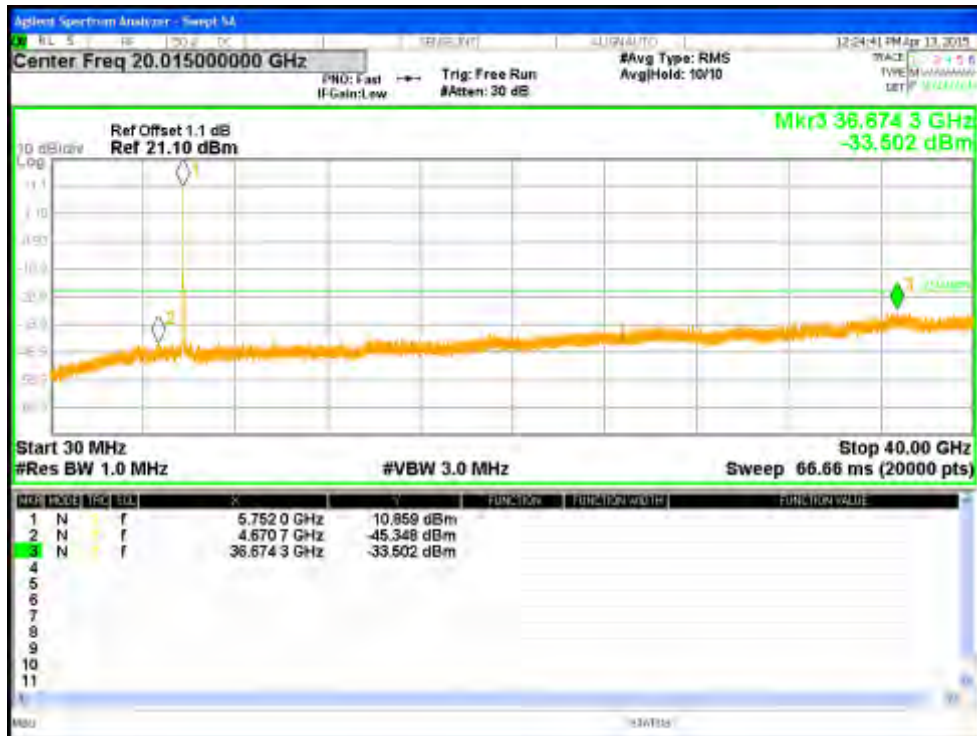
Figure 146: Undesirable Emission for 802.11a-6Mbps at 5745 MHz, Chain 0
