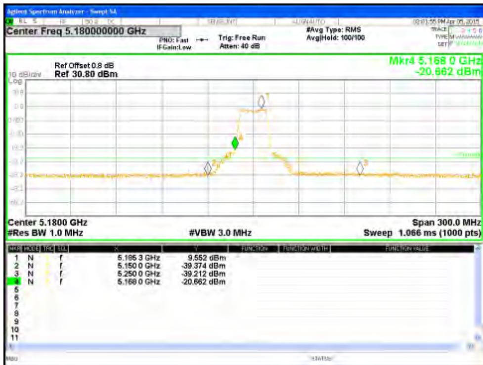
Figure 119: Measured Bandedge for VHT20-Nss2 MCS0 at 5180 MHz, Chain 1
