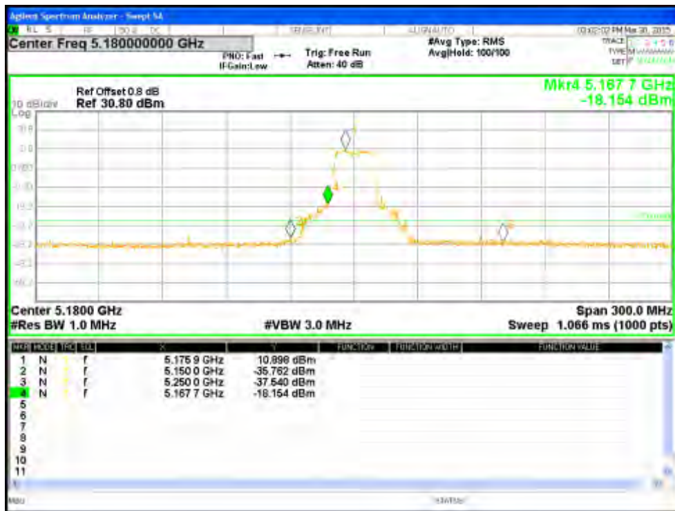
Figure 109: Measured Bandedge for HT20-MCS8 at 5180 MHz, Chain 0
