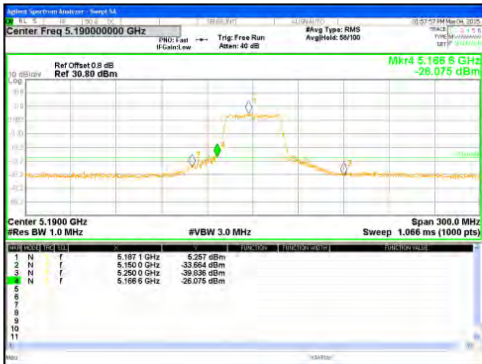
Figure 131: Measured Bandedge for VHT40-Nss1 MCS0 at 5190 MHz, Chain 1
