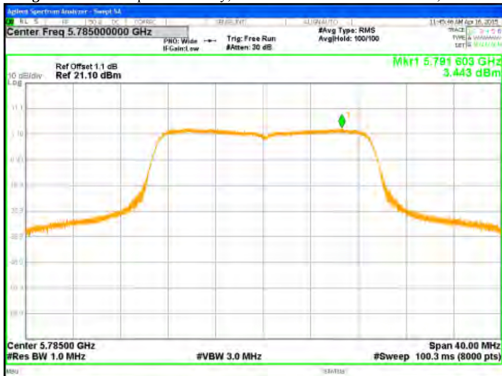
Figure 88: Power Spectral Density, 5785 MHz at VHT20 Nss2 MCS0, Chain 0
