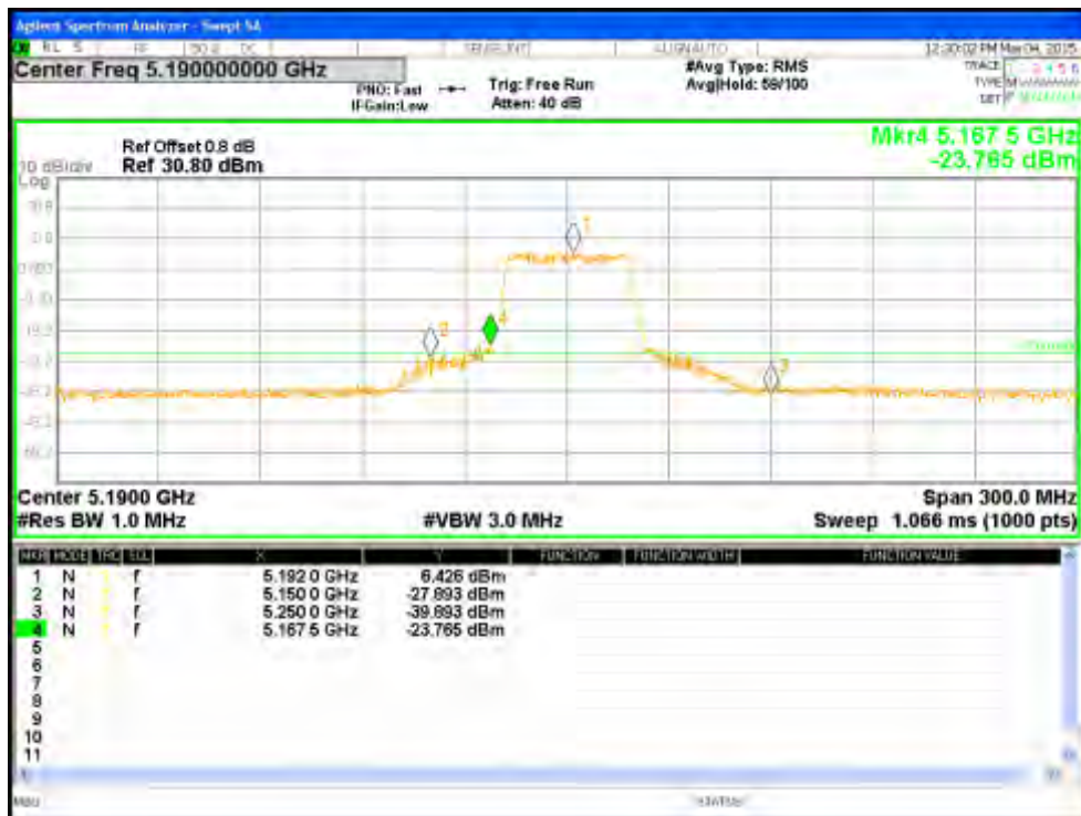
Figure 125: Measured Bandedge for HT40-MCS8 at 5190 MHz, Chain 0
