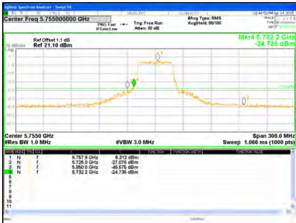
Figure 175: Measured Bandedge for VHT40-Nss1 MCS0 at 5755 MHz, Chain 1
