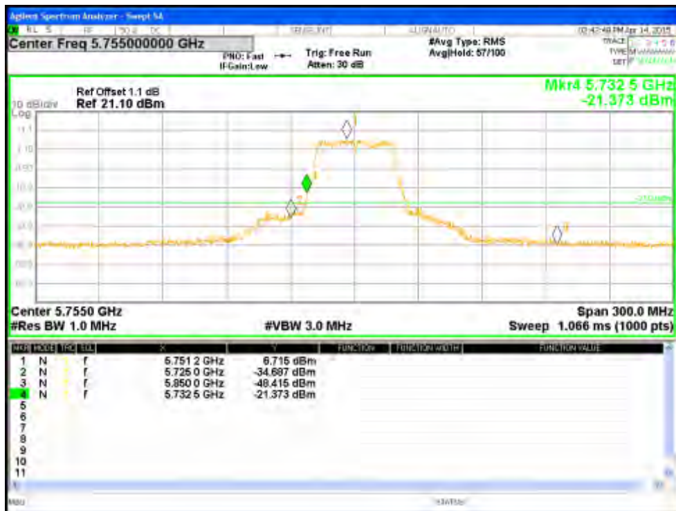
Figure 171: Measured Bandedge for HT40-MCS8 at 5755 MHz, Chain 1
