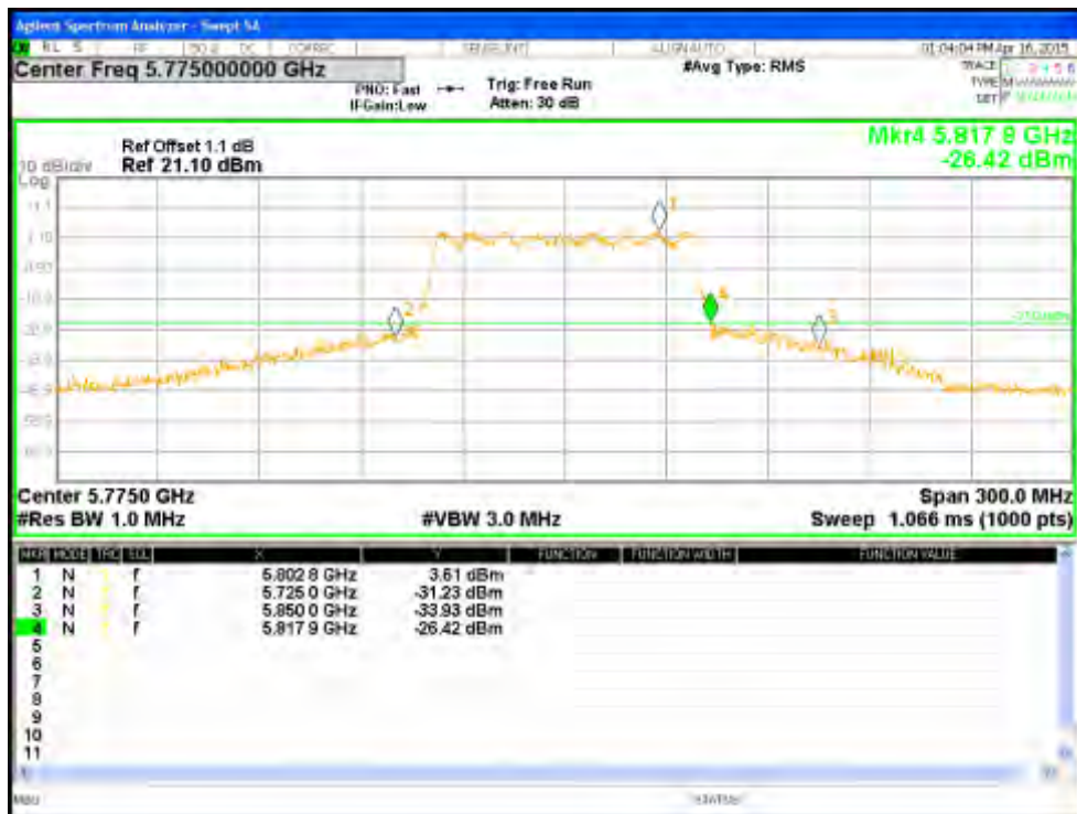
Figure 183: Measured Bandedge for VHT80-Nss1 MCS0 at 5775 MHz, Chain 1
