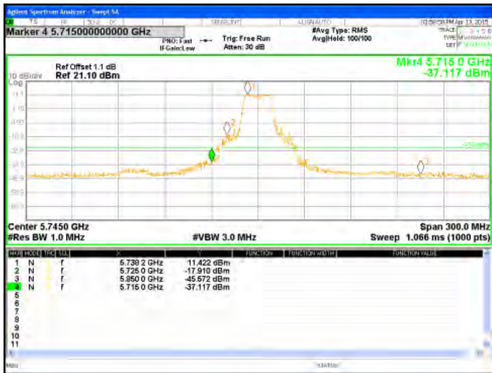
Figure 151: Measured Bandedge for HT20-MCS0 at 5745 MHz, Chain 1
