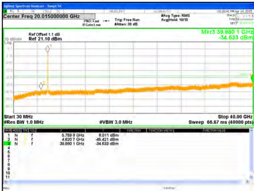
Figure 174: Undesirable Emission for VHT40-Nss1 MCS0 at 5755 MHz, Chain 0
