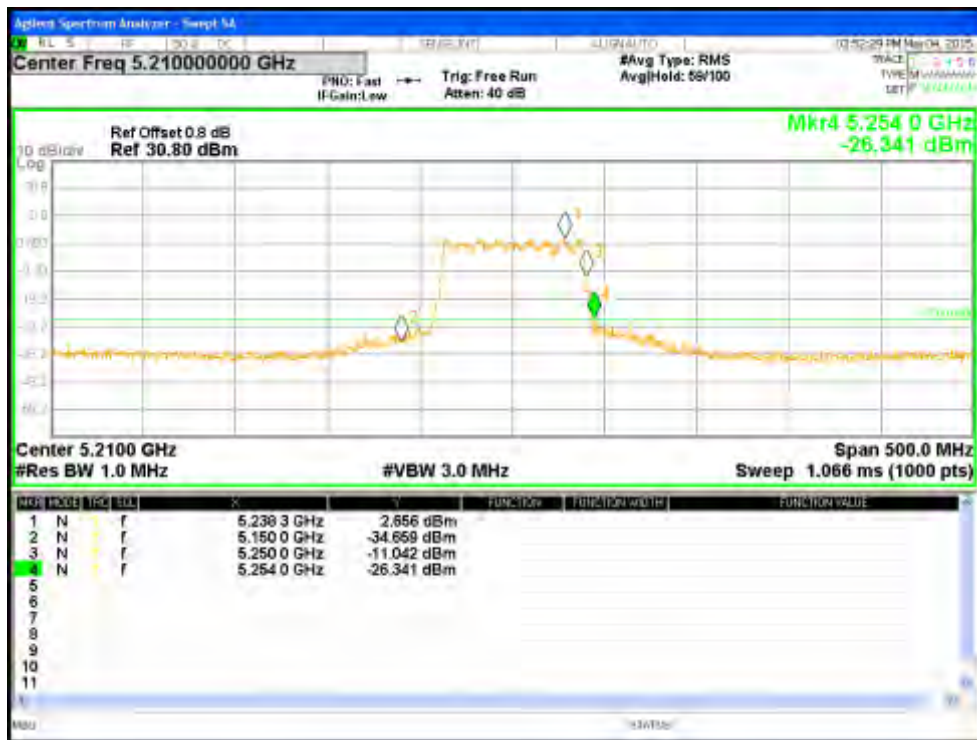
Figure 139: Measured Bandedge for VHT80-Nss1 MCS0 at 5190 MHz, Chain 1
