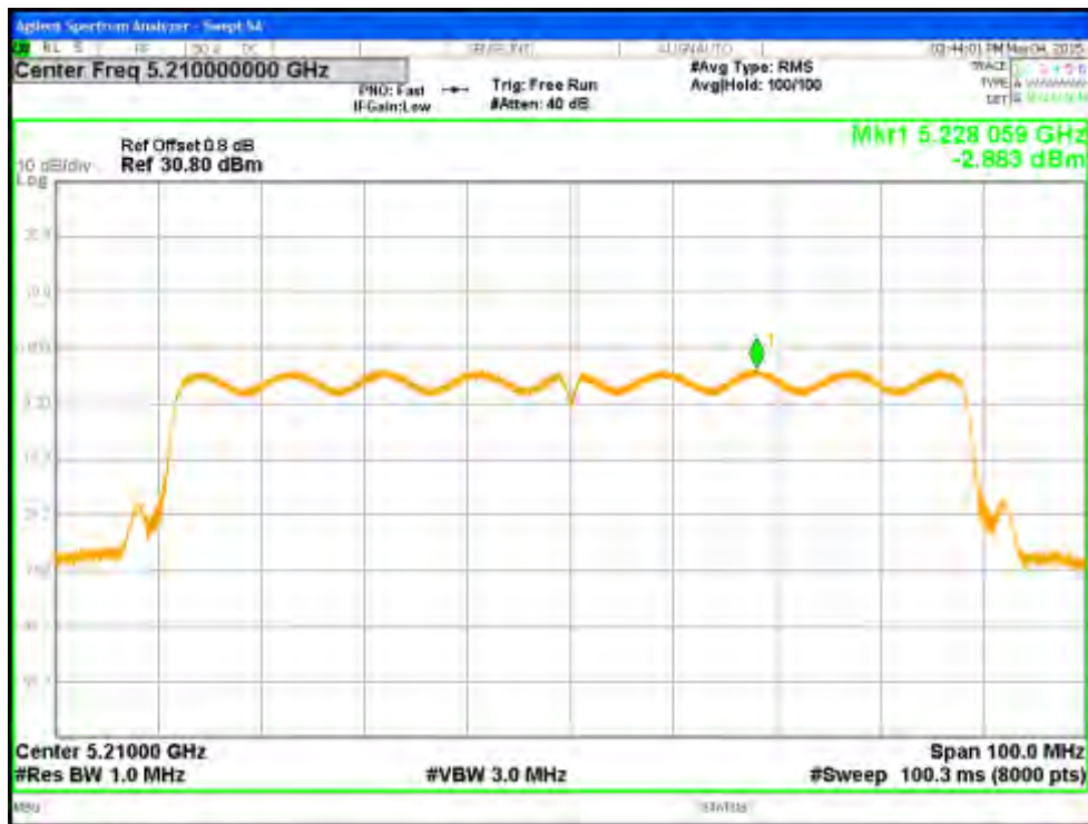
Figure 97: Power Spectral Density, 5210 MHz at VHT80 Nss1 MCS0, Chain 0
