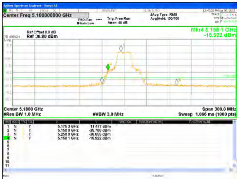
Figure 115: Measured Bandedge for VHT20-Nss1 MCS0 at 5180 MHz, Chain 1
