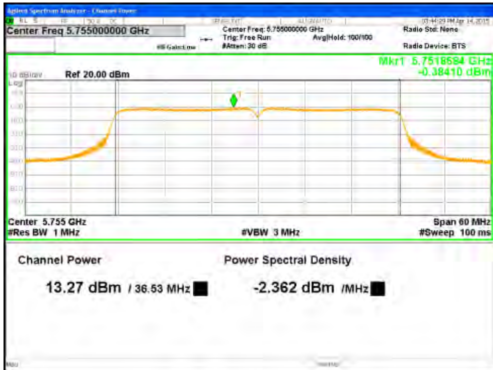
Figure 26: Maximum Transmitted Power, 5755 MHz at VHT40 Nss1 MCS0, Chain 1
