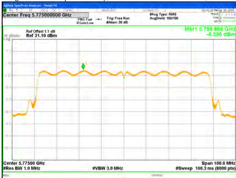
Figure 100: Power Spectral Density, 5775 MHz at VHT80 Nss2 MCS0, Chain 0
