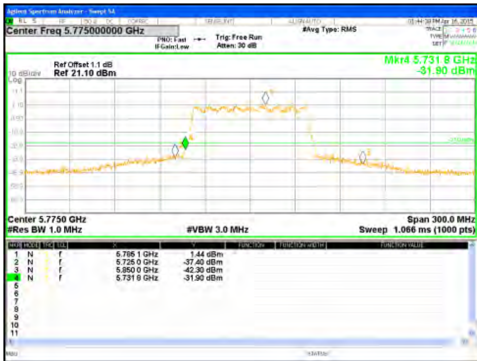
Figure 187: Measured Bandedge for VHT80-Nss2 MCS0 at 5775 MHz, Chain 1
