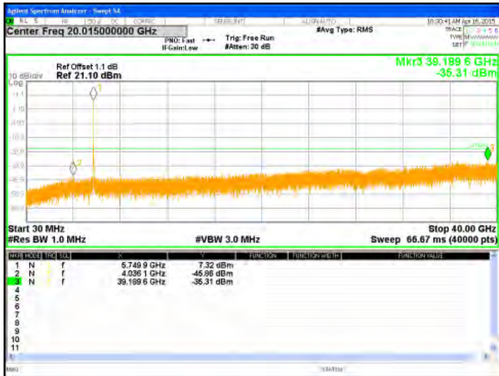
Figure 160: Undesirable Emission for VHT20-Nss1 MCS0 at 5745 MHz, Chain 1
