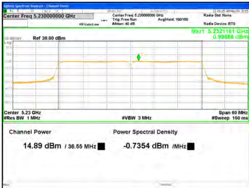
Figure 17: Maximum Transmitted Power, 5230 MHz at HT40 MCS0, Chain 0
