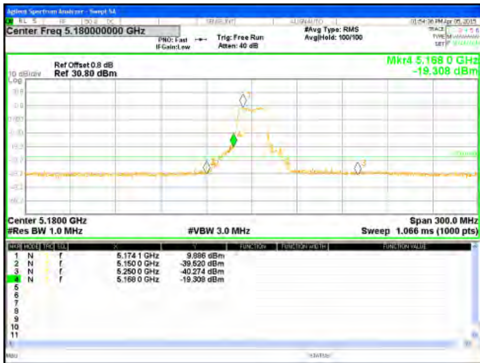
Figure 117: Measured Bandedge for VHT20-Nss2 MCS0 at 5180 MHz, Chain 0
