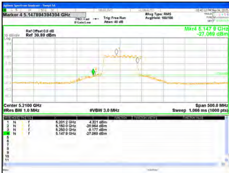
Figure 137: Measured Bandedge for VHT80-Nss1 MCS0 at 5190 MHz, Chain 0
