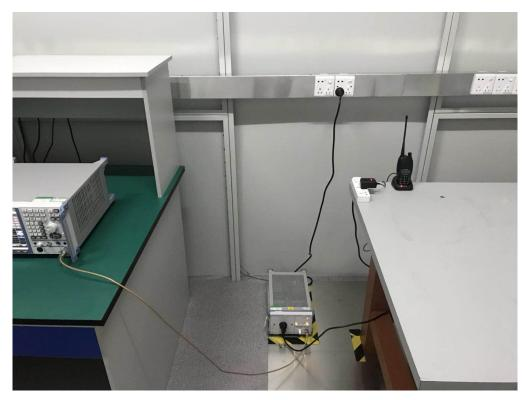
RADIATED EMISSION TEST SETUP
