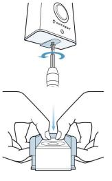
A Use the included Philips head screwdriver to remove the bracket screw from the doorbell.
