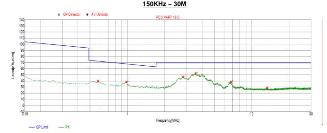
Level Factor Limit Margin NO. Freq.[MHz] Remark [dBµV/m] [dB] [dBµV/m] [dB] peak 1 0.5829 39.49 19.71 72.30 -32.81 2 0.9829 38.32 19.94 67.77 -29.45 peak peak 3 2.8159 46.65 20.06 69.50 -22.85 -17.10 peak 4 3.5443 52.40 20.11 69.50 5 6.8132 38.12 20.25 69.50 -31.38 peak 13.2584 20.29 69.50 -40.88 peak 6 28.62
