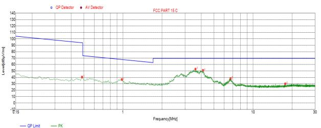
Level Factor Limit Margin NO. Freq.[MHz] Remark [dBµV/m] [dB] [dBµV/m] [dB] peak 1 0.4844 40.48 19.60 93.90 -53.42 2 0.9799 36.66 19.94 67.80 -31.14 peak peak 3 3.6100 52.90 20.11 69.50 -16.60 peak 4 4.1234 51.01 20.14 69.50 -18.49 5 6.7177 38.09 20.25 69.50 -31.41 peak 17.7006 30.00 69.50 -39.50 peak 6 21.42
