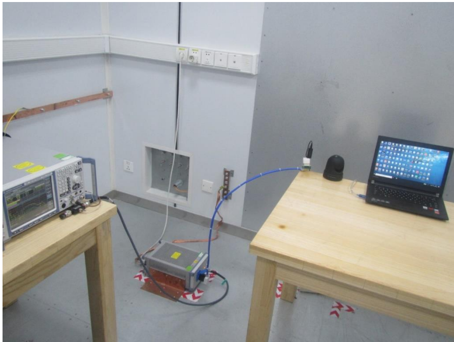
POWERLINE CONDUCTED EMISSIONS MEASUREMENT SETUP
