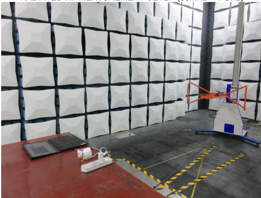
RADIATED RF MEASUREMENT SETUP (30MHz ~ 1 GHz)
