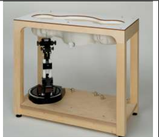
Fig. 8.7 Photo of SAM Twin Phantom
