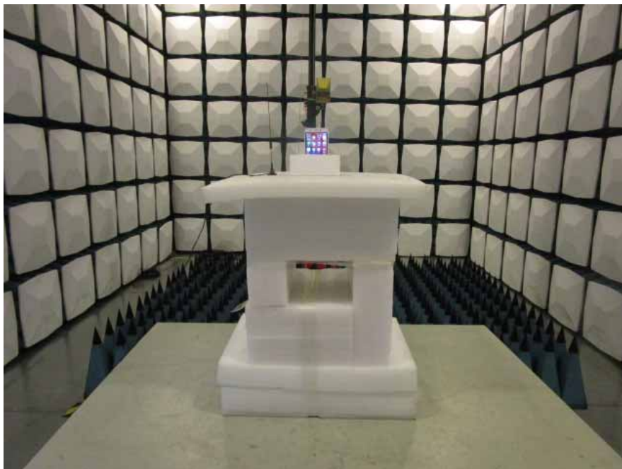
Radiated Emission View---Above 1GHz
