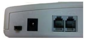
There are two communication portals at the back of the terminal. You can connect desktop phones with our terminal. It's very easy to connect the phone and terminal, just need a common communication cable.
