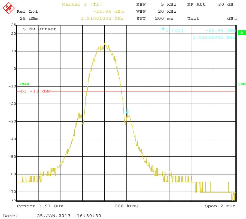
**WCDMA(QPSK) Mode****Cellular Band, Left Band Edge**
