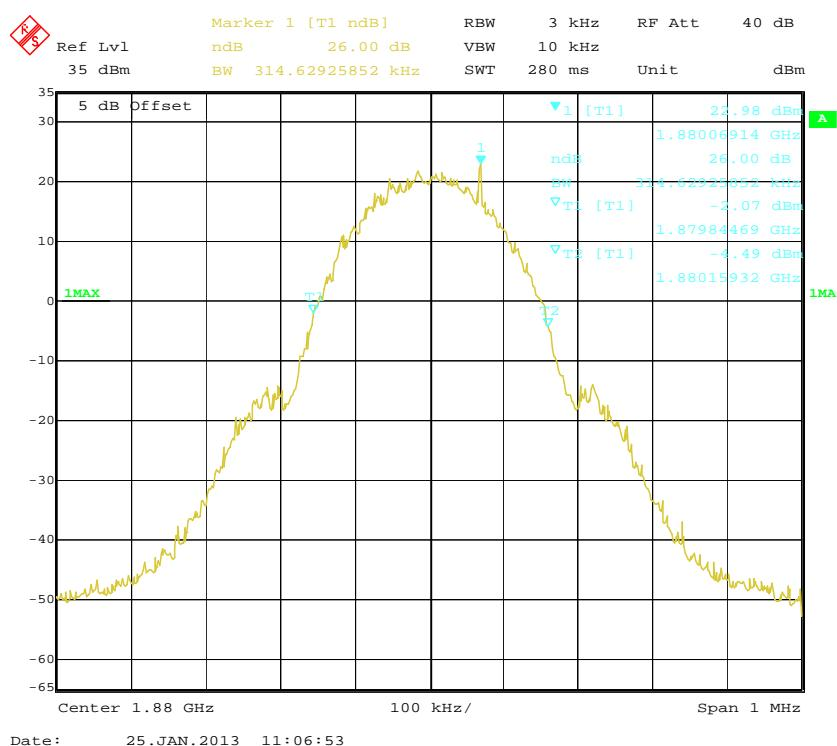
**99% Occupied Bandwidth for EGPRS (8PSK) Mode**
