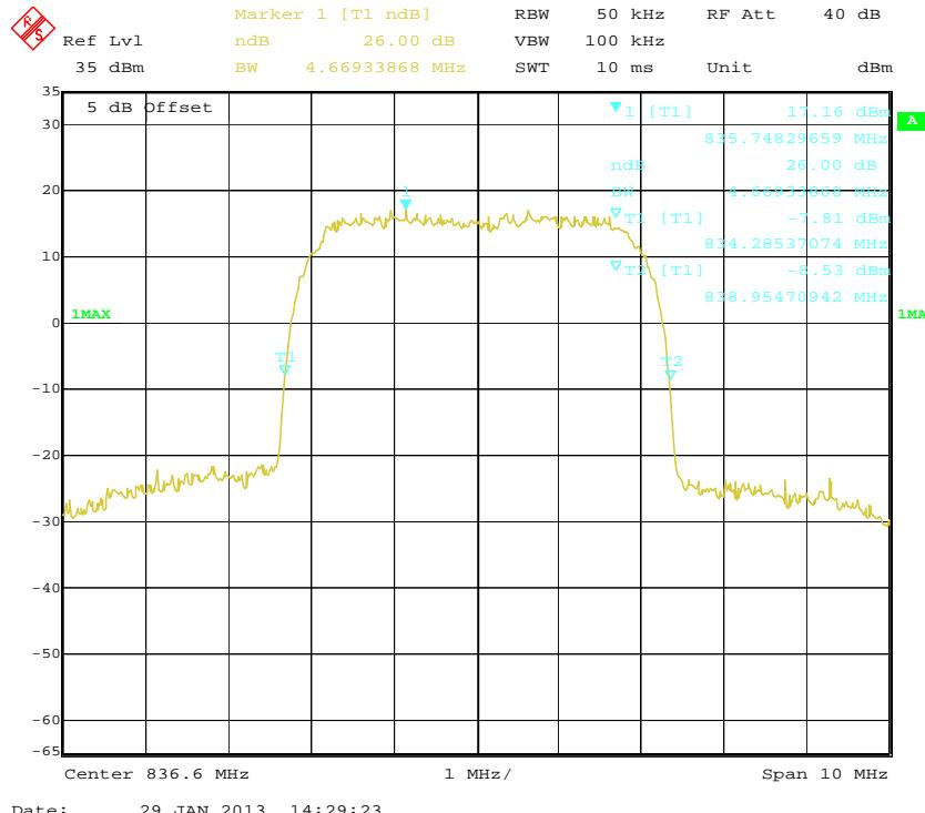
**PCS Band (Part 24E)****99% Occupied Bandwidth for GSM (GMSK) Mode**
