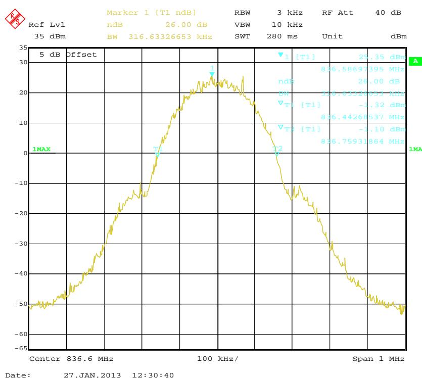
**99% Occupied Bandwidth for EGPRS (8PSK) Mode**
