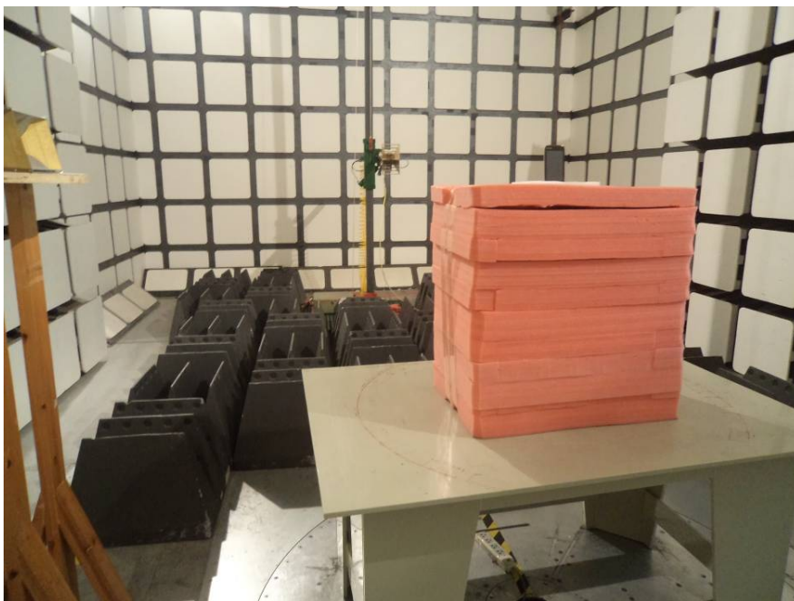
Radiated Emissions Test View (Above 1 GHz)
