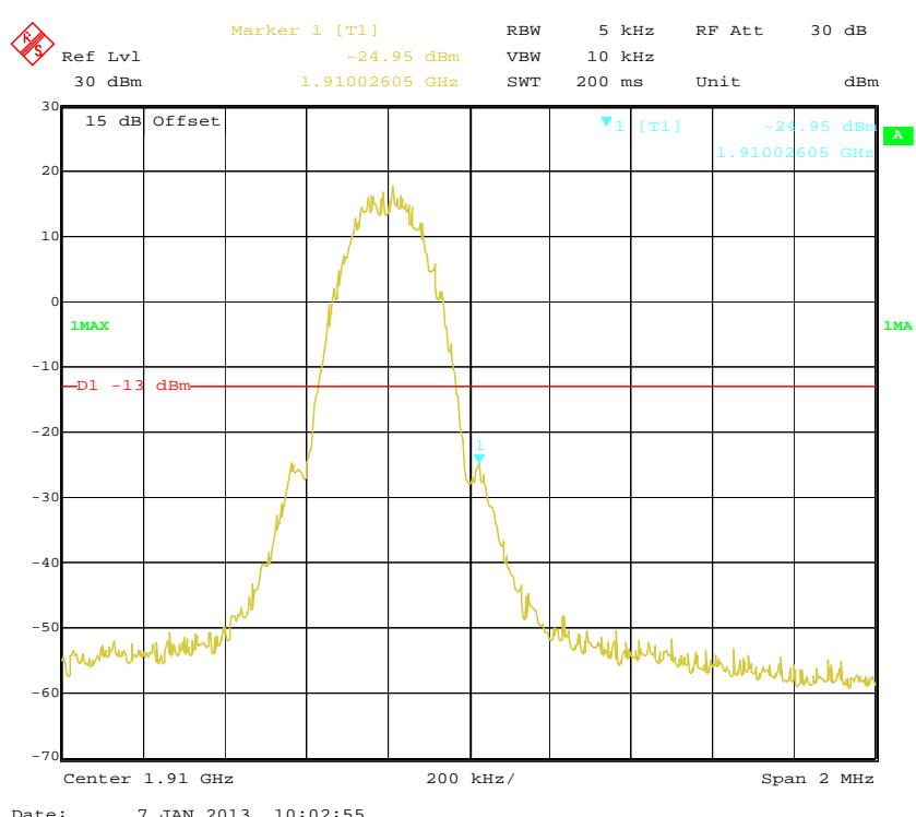
**EGPRS (8PSK) Mode****Cellular Band, Left Band Edge**
