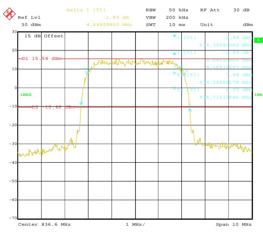
**Bandwidth for HSDPA (16QMA) Mode**
