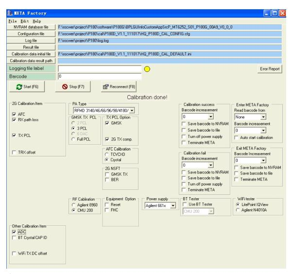
⑥ Once the button is clicked, the CMU will be checking various parameters automatically( e.g. RSSI, Output Power, AFC,etc.) and set different parameters for the mobile phone accordingly(e.g. Gain, Output power, etc.)
