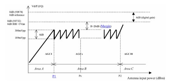
**Area A:** The total gain of the receiver is maximum and constant for all RF input power below P1; the I/Q amplitude increases linearly versus the RF input power until it reaches 300mVpp. The AGC is set to maximum gain AGC1.
