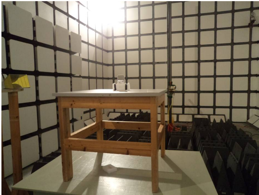
Above 1GHz: Radiated Emissions - Rear View
