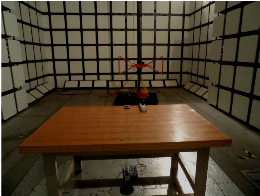
Below 1 GHz: Radiated Emissions - Rear View
