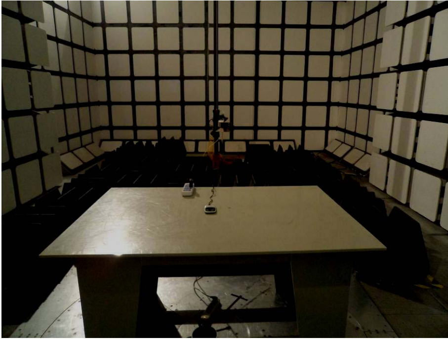
Above 1 GHz: Radiated Emissions - Rear View
