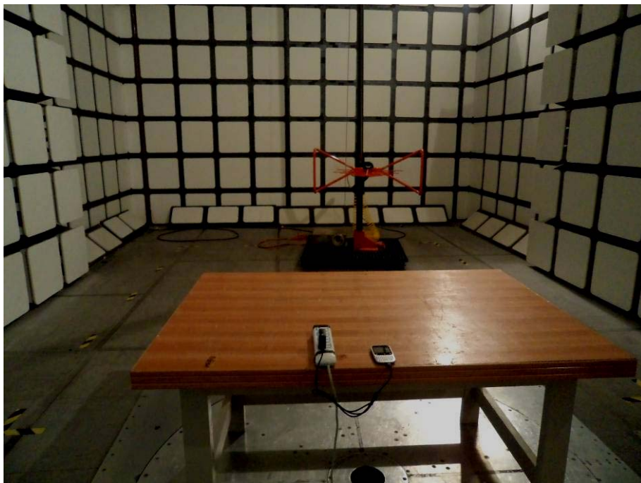
Below 1 GHz: Radiated Emissions - Rear View
