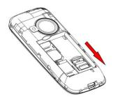
4) With the metallic contacts of the battery facing the metallic contacts in the battery slot, press the battery down until it locks into place, then fix its back cover.
