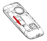
3) To install the T-Flash card, open its latch, place its indented side downward, insert the card into the card slot, and then close the latch.
