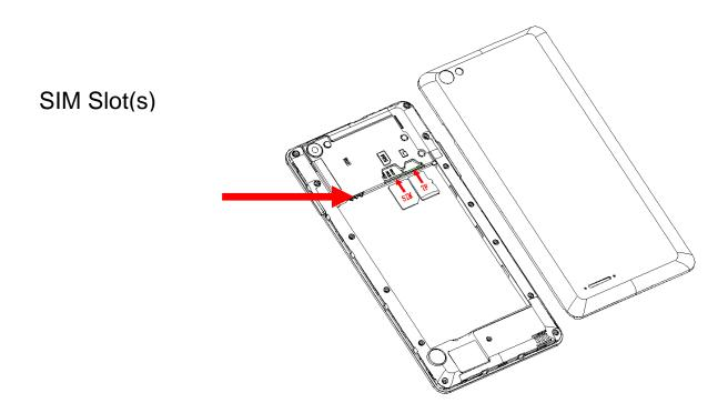
3. Replace the rear cover of the mobile phone and power on.
