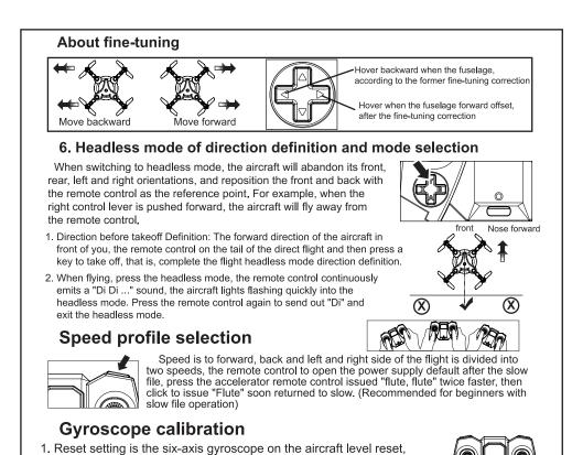
2. Before the operation of the aircraft in a horizontal position (if the tripod deformation, the aircraft four corners have a high and low reset after the aircraft take-off will affect the stability) and then the remote control as shown below down two seconds after the remote control Issued a "flute" two sound, the aircraft quickly within the light a few times, said the reset is set.
