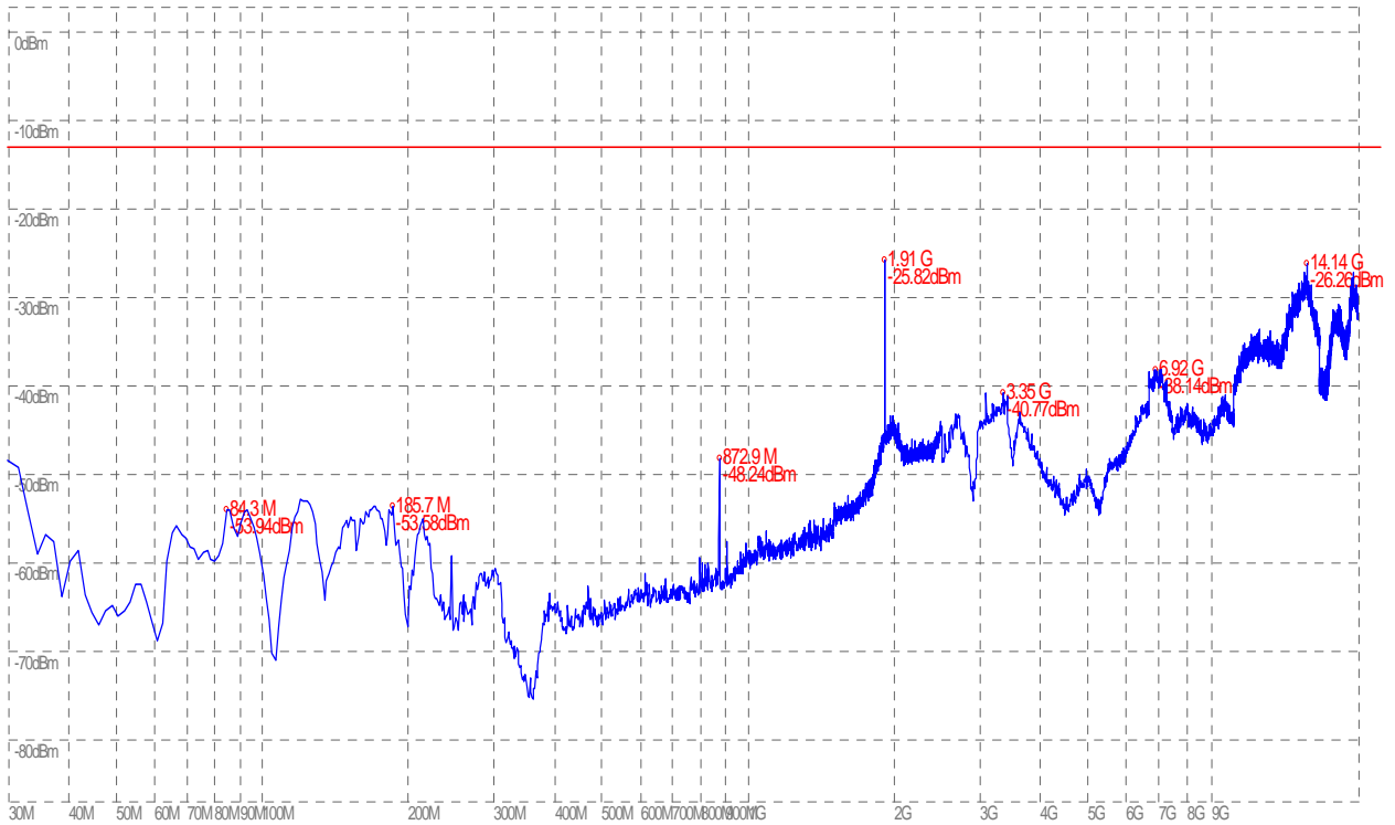
(Plot B 6: EGPRS 1900MHz Channel = 810, Test Antenna Vertical)
