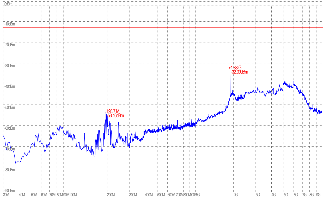
(Plot D.3: WCDMA 1900MHz Channel = 9400, Test Antenna Horizontal)
