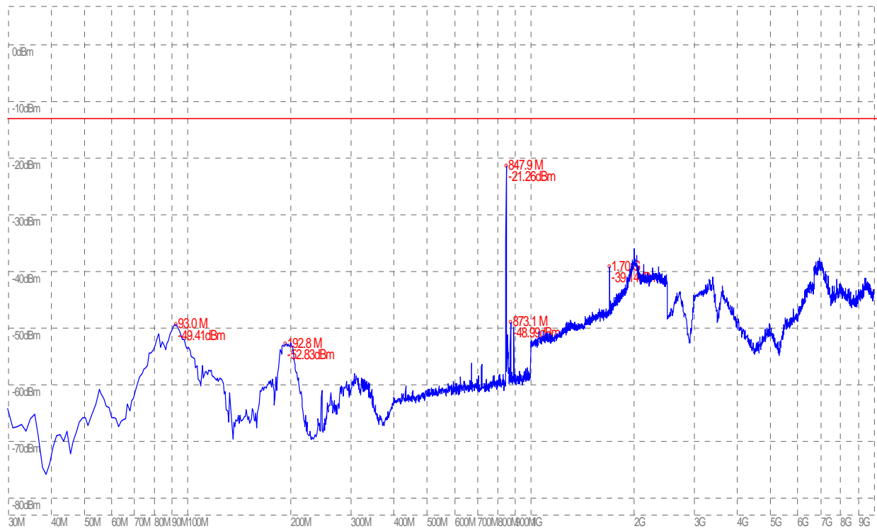
(Plot A.5: EGPRS 850MHz Channel = 251, Test Antenna Horizontal)
