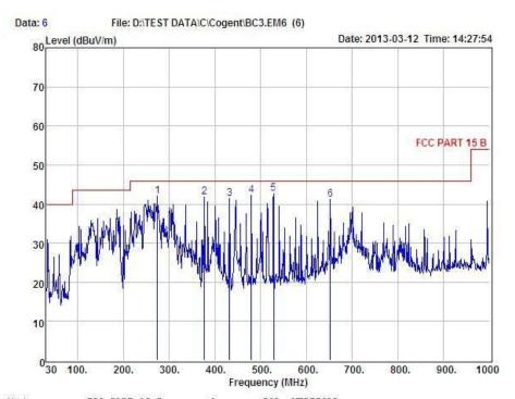
Condition : FCC PART 15 B 3m POL: VERTICAL EUT : BlueCheck III mobile single finger capture device
