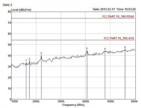
: FCC PART 15\_18G PEAK 3m POL: HORIZONTAL : BlueCheck III mobile single finger capture device : BC3 Condition EUI
