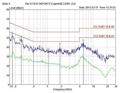
Condition : FCC PART 15 B QP POL: LINE Temp: Hum: EUT : BlueCheck III mobile single finger capture device
