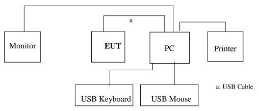
EUT: BlueCheck III mobile single finger capture device, incorporating the cogent CSD330, without membrane at 500ppi
