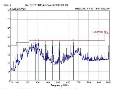
Condition : FCC PART 15 B 3m POL: HORIZONTAL EUT : BlueCheck III mobile single finger capture device
