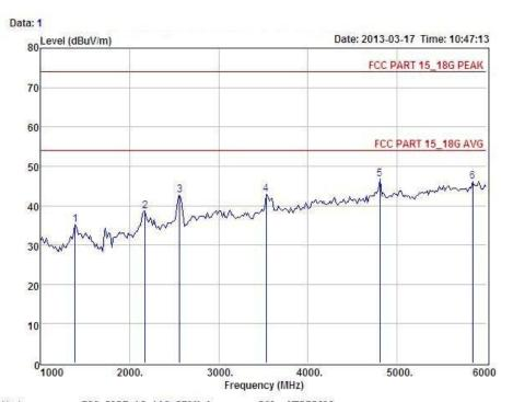
: FCC PART 15\_18G PEAK 3m POL: VERTICAL : BlueCheck III mobile single finger capture device : BC3 Condition EUT
