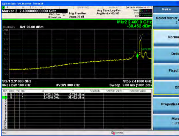
(8DPSK): Band Edge-Low Channel (Hopping Mode)
