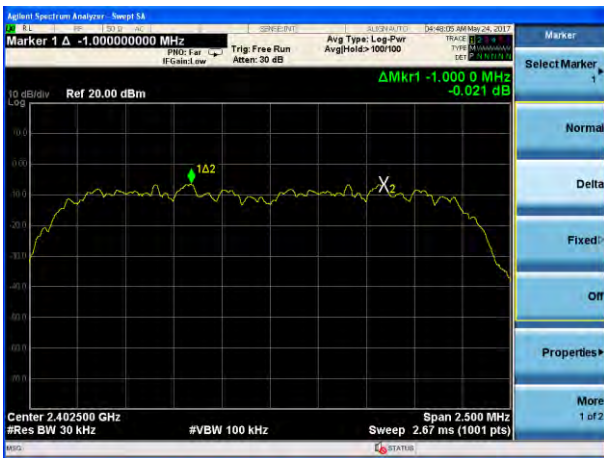
(3Mbps) Channel Separation plot on channel 39-40
