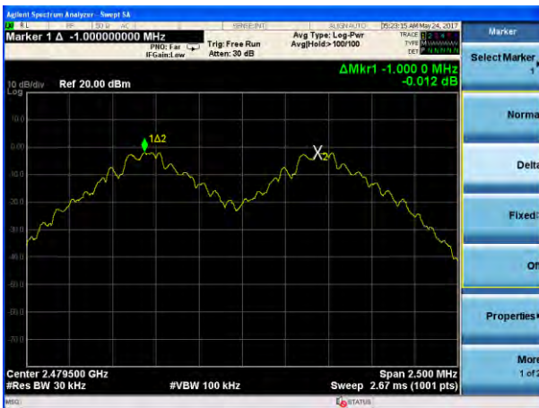
(1Mbps) Channel Separation plot on channel 77-78
