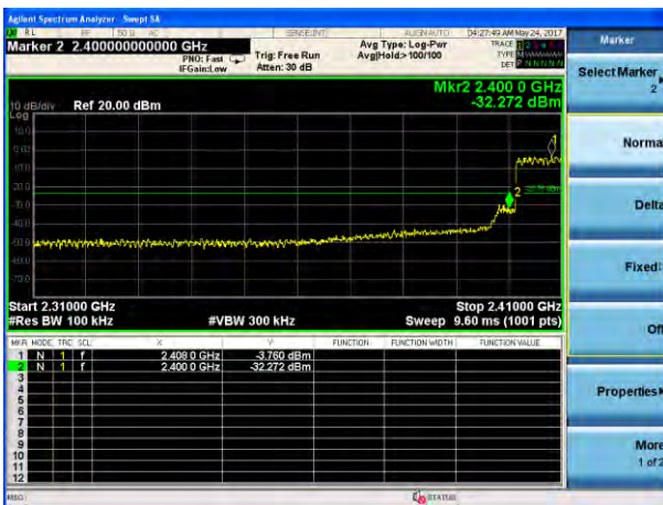
( \pi /4-DQPSK): Band Edge-Low Channel (Hopping Mode)
