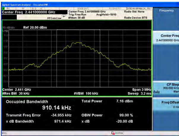
20dB Bandwidth plot on channel 78 (1Mbps)
