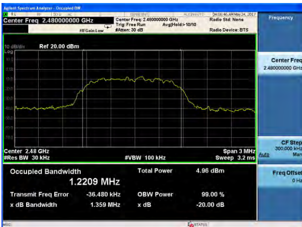
20dB Bandwidth plot on channel 78 (3Mbps)
