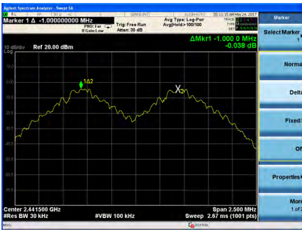
(1Mbps) Channel Separation plot on channel 77-78
