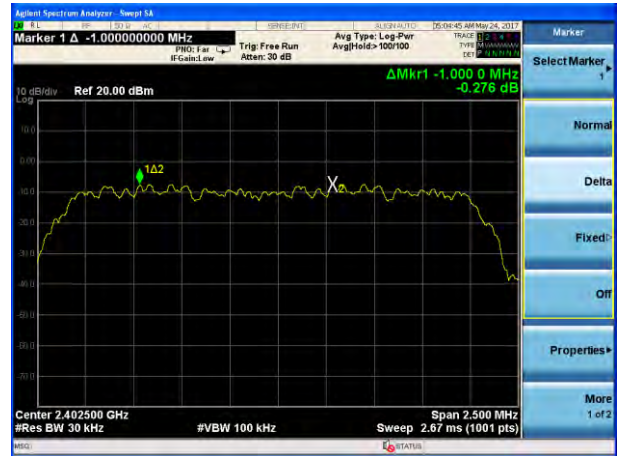
(2Mbps) Channel Separation plot on channel 39-40
