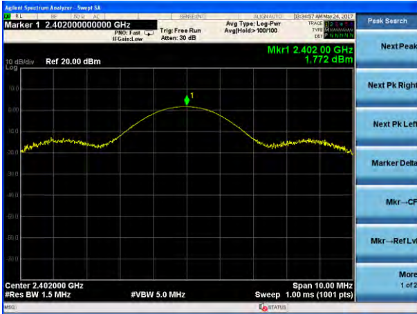
Peak output Power plot on channel 39 (3Mbps)
