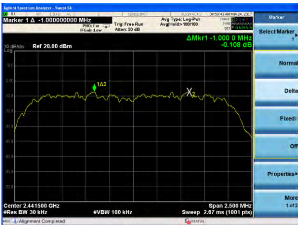
(3Mbps) Channel Separation plot on channel 77-78
