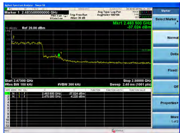
( \pi /4-DQPSK): Band Edge-High Channel (Hopping Mode)
