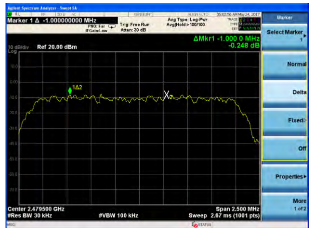
(2Mbps) Channel Separation plot on channel 77-78
