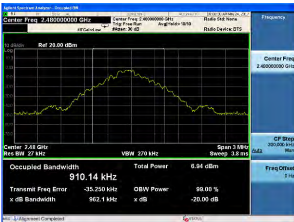
20dB Bandwidth plot on channel 78 (1Mbps)
