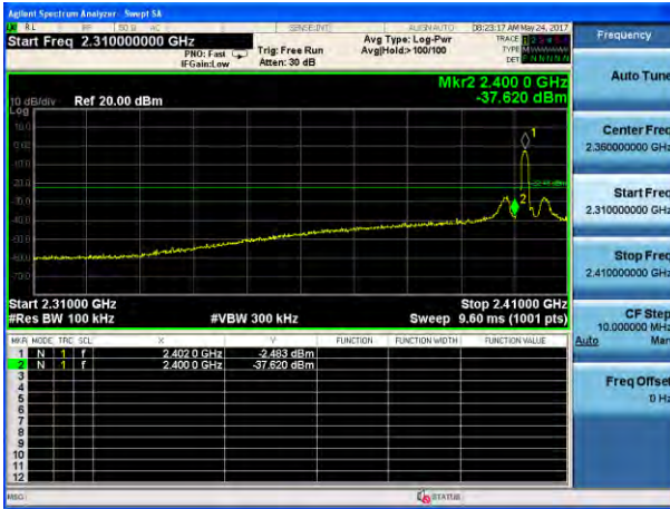
( \pi /4-DQPSK): Band Edge-Low Channel (Hopping Mode)
