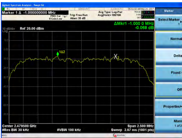
(3Mbps) Channel Separation plot on channel 77-78
