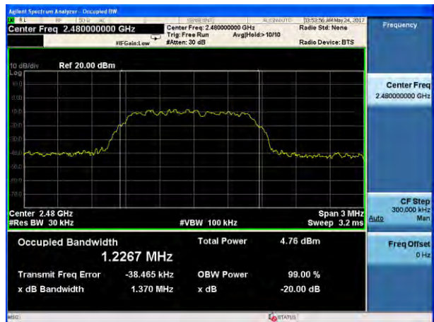
20dB Bandwidth plot on channel 78 (2Mbps)
