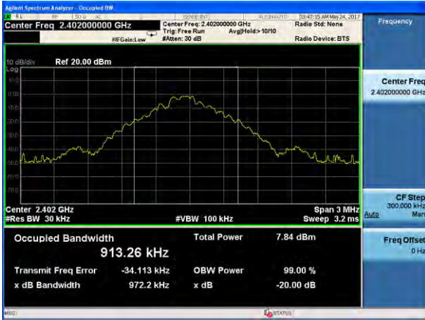
20dB Bandwidth plot on channel 39 (1Mbps)
