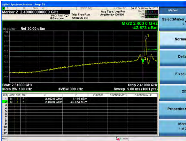
(GFSK): Band Edge-Low Channel (Hopping Mode)
