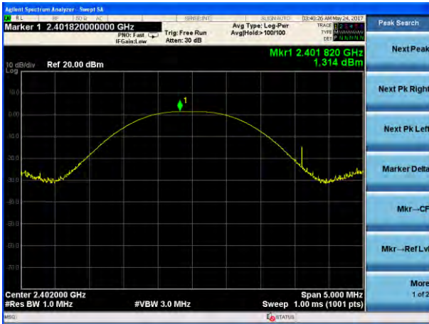
Peak output Power plot on channel 39 (1Mbps)
