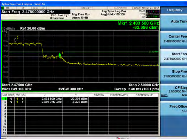
(8DPSK): Band Edge-High Channel (Hopping Mode)
