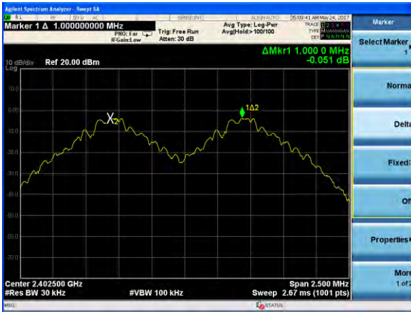
(1Mbps) Channel Separation plot on channel 39-40
