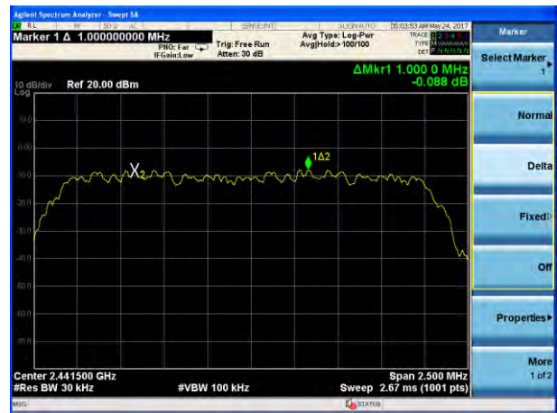
(2Mbps) Channel Separation plot on channel 77-78
