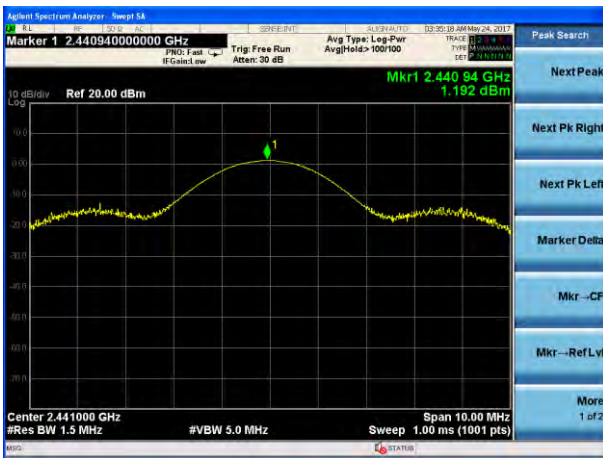
Peak output Power plot on channel 39 (3Mbps)
