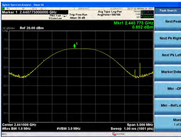
Peak output Power plot on channel 78 (1Mbps)
