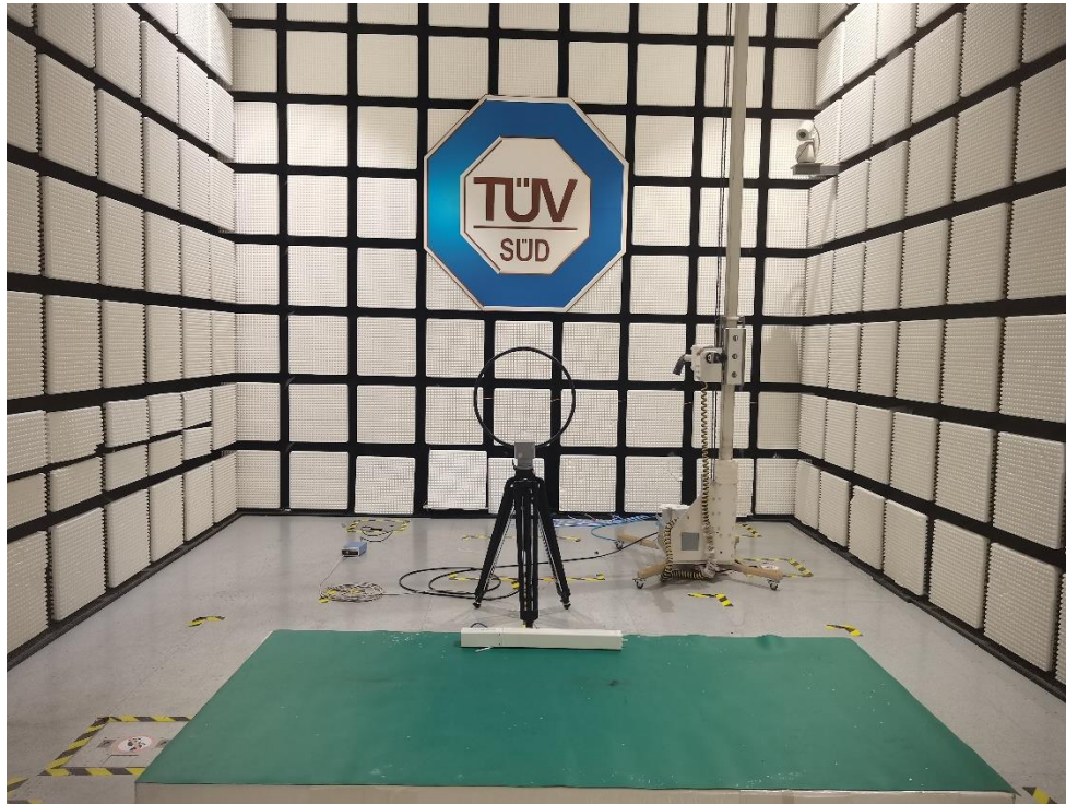
Radiated Emission Setup 9kHz ~ 30MHz
