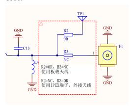
R2=0ohm & R3=NC, uses on board antenna R2=NC & R3=0ohm, uses external antenna via IPEX port
