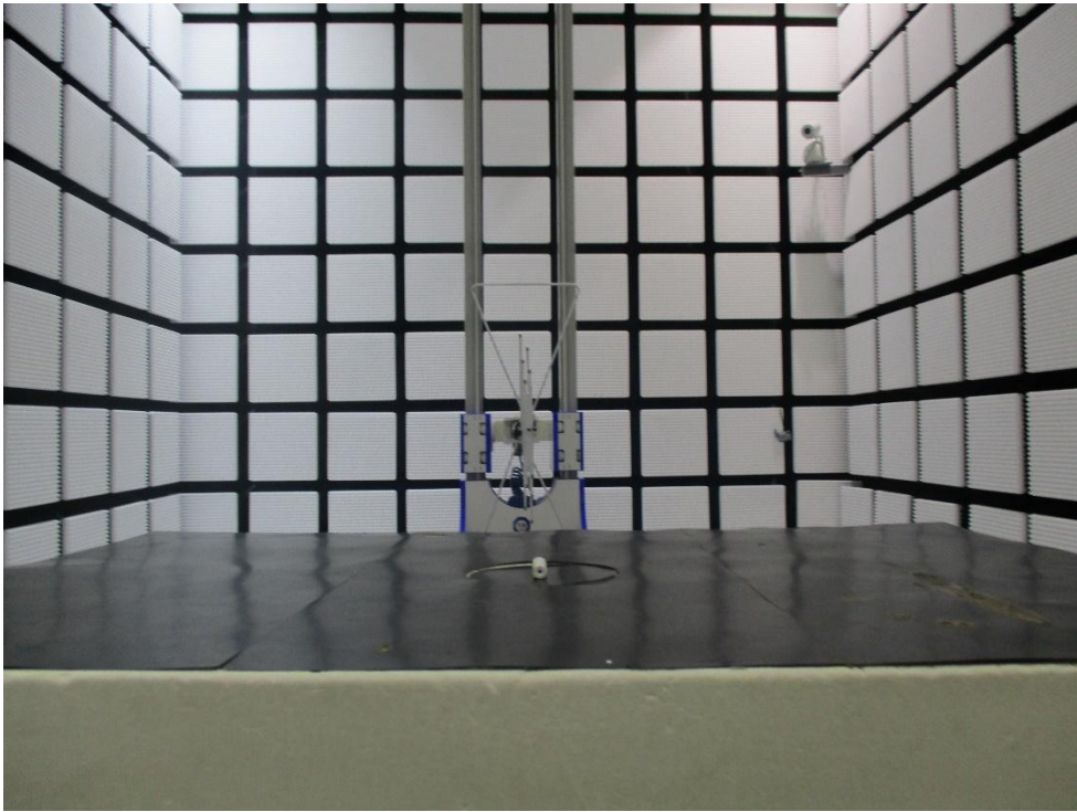
Radiated Emission Test above 1GHz
