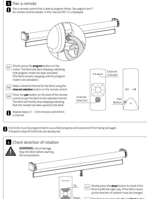
4.2 Simultaneously press the **up** and **down** button to change the direction of rotation.
