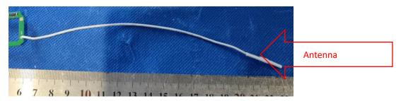
Antenna transmission frequency: 433.92MHz
