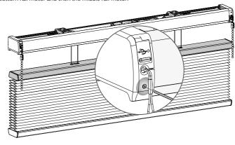
Pair the middle rail motor to an empty channel on the remote. (see step 5)
