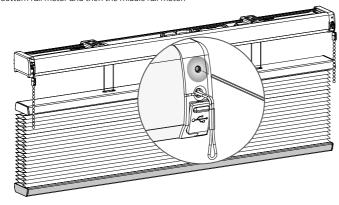
Pair the bottom rail motor to an empty channel on the remote. (see step 5)
