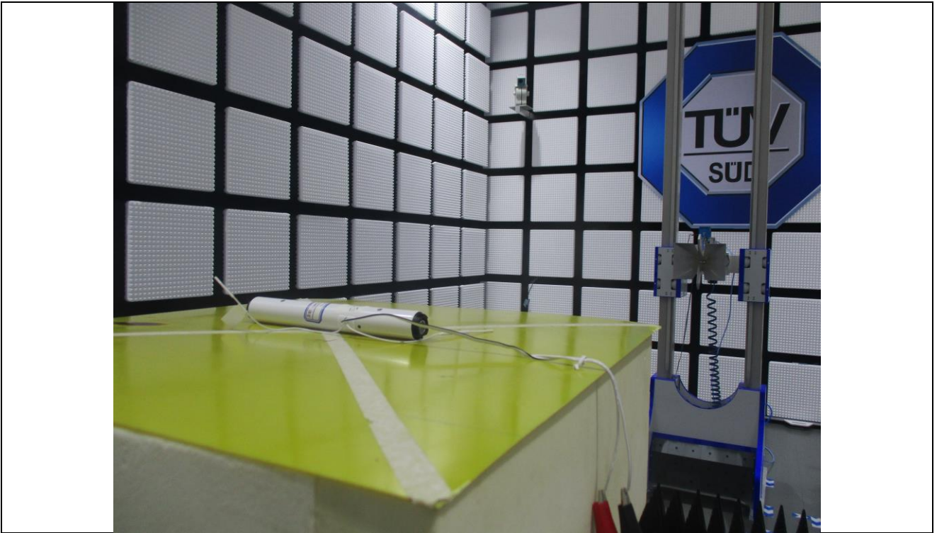
Radiated Emission test (1000MHz to 18000MHz)
