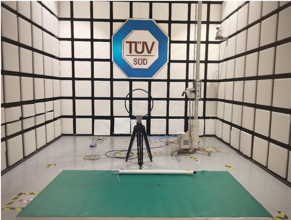
Radiated Emission Setup 9kHz ~ 30MHz
