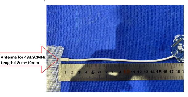
Antenna transmission frequency: 433.92MHz
