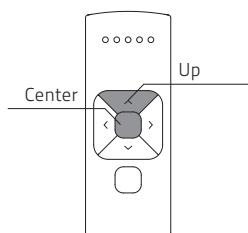
8.1 Simultaneously hold the **center** and the **up** button until the blind stops stepping and starts stepping again.
