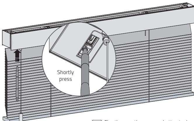
**12.1** Shortly press the program button to de-activate program mode. The blind stops stepping and can be operated.
