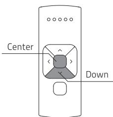
**10.1** Simultaneously hold the **center** and the **down** button until the blind stops stepping and starts stepping again.
