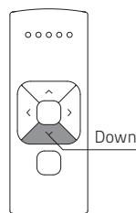
7.1 Press and hold the **down** button until the blind reaches the desired bottom position.
