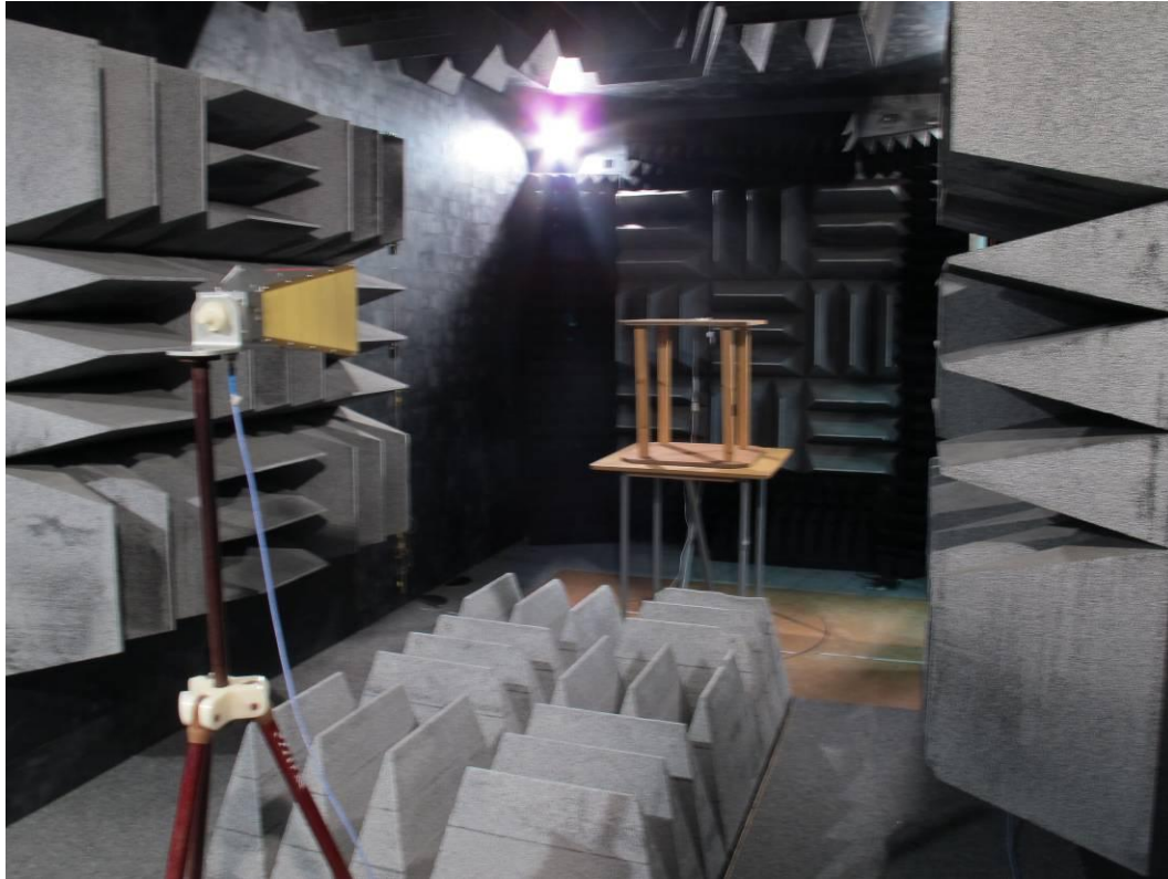
Photograph 2: - Test setup radiated emissions 1 – 18 GHz
