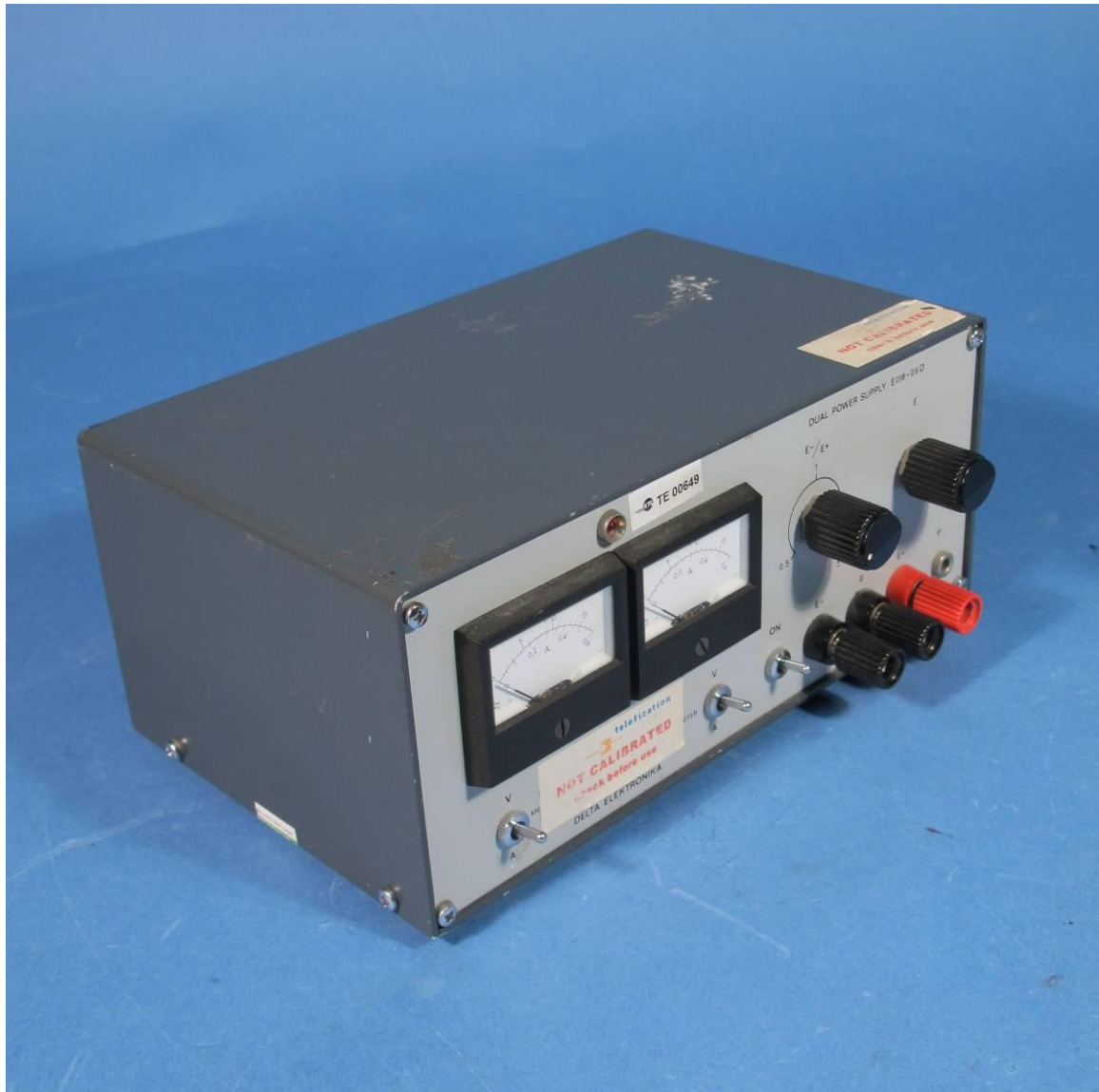
Photograph 3: - AC mains power supply, type E018-06D
