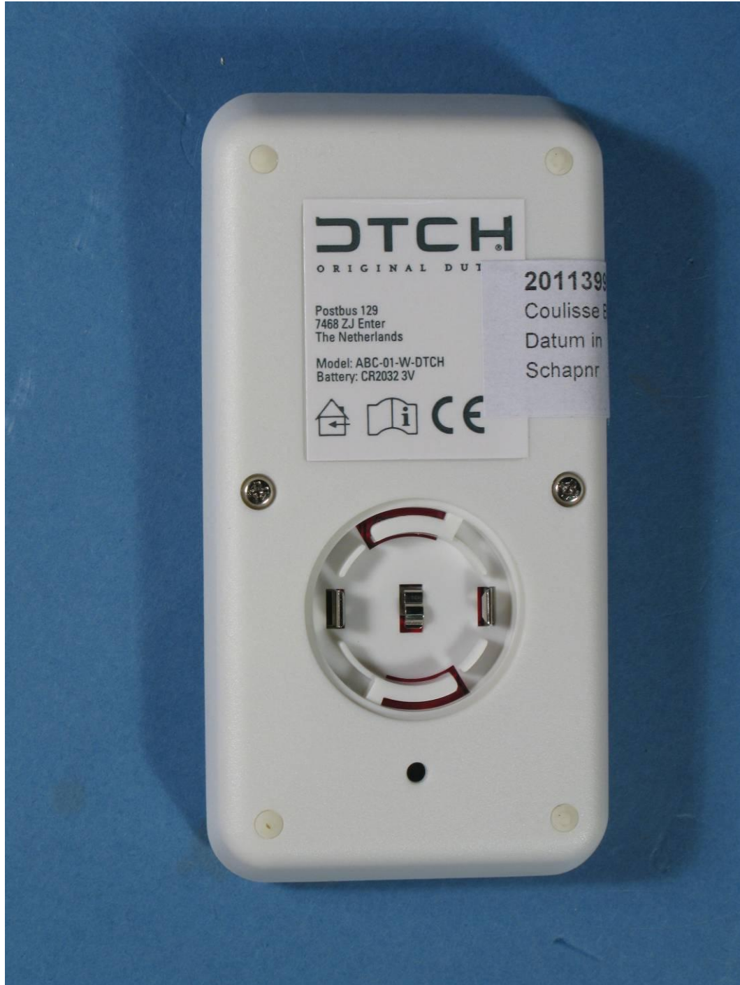
Photograph 6: - ABC-01-DTCH, remote control, battery compartment
