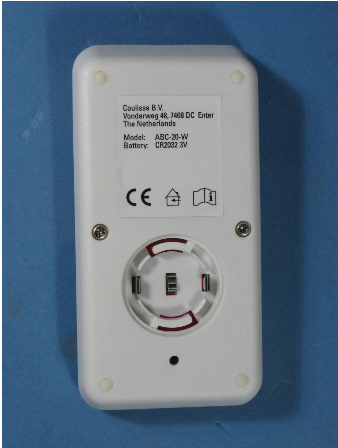
Photograph 9: - ABC20, remote control, battery compartment
