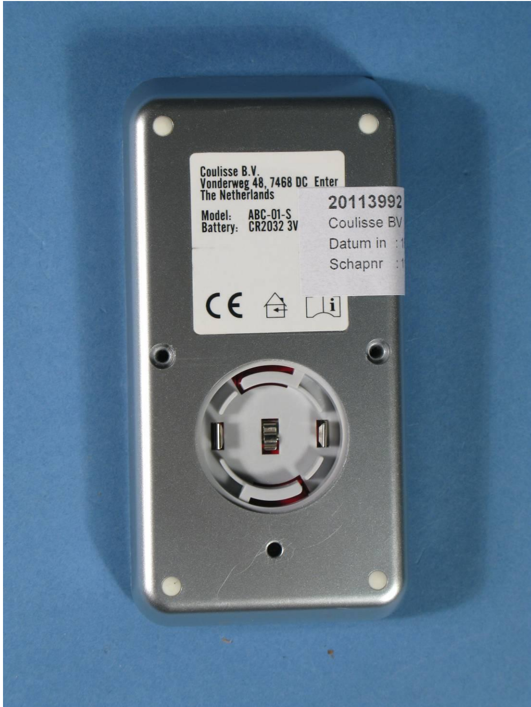
Photograph 3: - ABC-01, remote control, battery compartment
