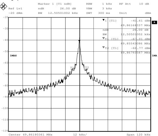
26dB bandwidth lower frequency: 49.85543086MHz 26dB bandwidth upper frequency: 49.86793587MHz
