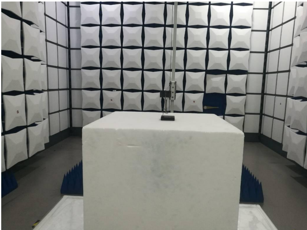
FCC RADIATED EMISSION TEST SETUP ABOVE 1GHZ
