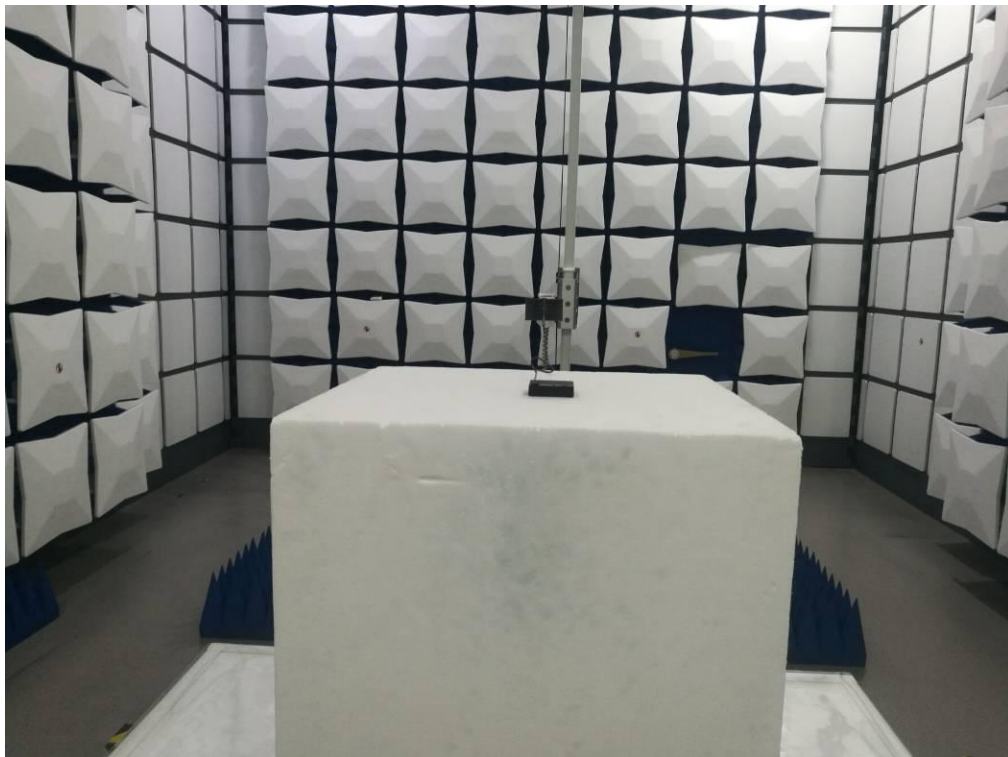
FCC RADIATED EMISSION TEST SETUP ABOVE 1GHZ
