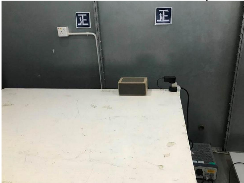
Measurement of Conducted Emission Test Set Up
