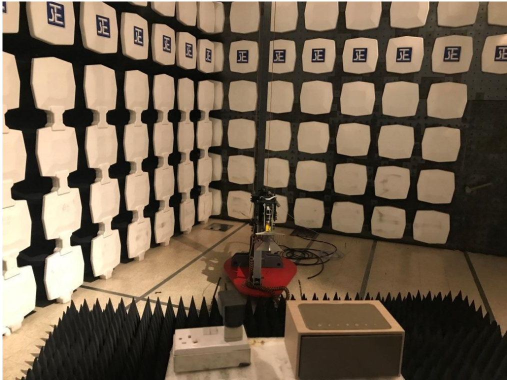
Measurement of Radiated Emission Test Set Up (Above 1000MHz)
