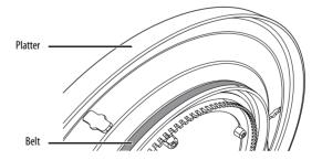
1 Make sure that the belt is not twisted, then use your thumb to stretch the belt until it reaches the round hole in the platter.
