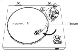
7 Push the tone arm lifter backward to lower the tone arm so that the stylus touches the record and starts to play.
