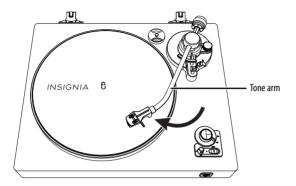
5 Turn the counterweight so that the tone arm is horizontal. You can move the counterweight forward or backward on the tone arm.
