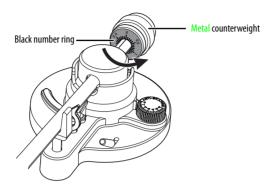
**8** Hold both the metal counterweight and black number ring together and rotate them counter-clockwise so that 2.5 on the dial is in the 12 o'clock position. This adjustment sets the tone arm to 2.5 grams of downward force (the recommended tracking weight) for this needle.
