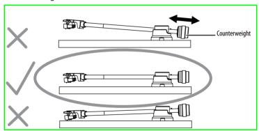
6 Hold the metal counterweight at the back of the tone arm.
