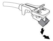
3 Push new stylus upwards until the tip locks into place.
