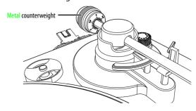
7 Hold the metal counterweight to keep it from moving, then carefully rotate the front black number ring so that 0 is in the 12 o'clock position.
