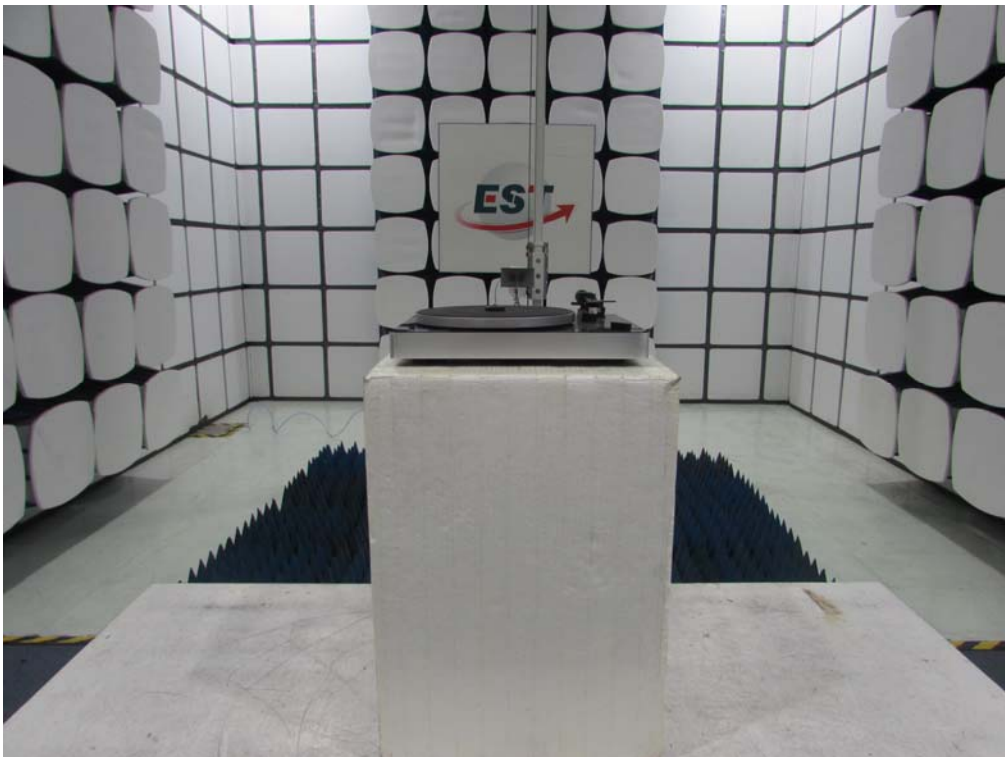
Radiated Test (Above 1GHz)
