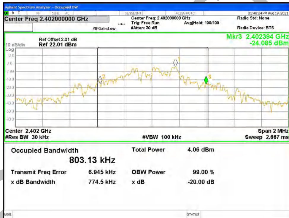
-20dB Bandwidth NVNT 1-DH1 2402MHz Ant1
