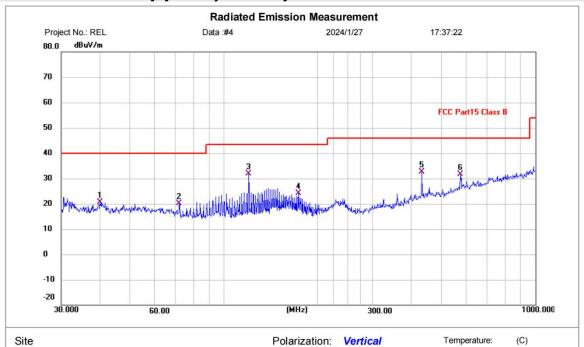
Limit: FCC Part15 Class B EUT: BLE Bluetooth module
