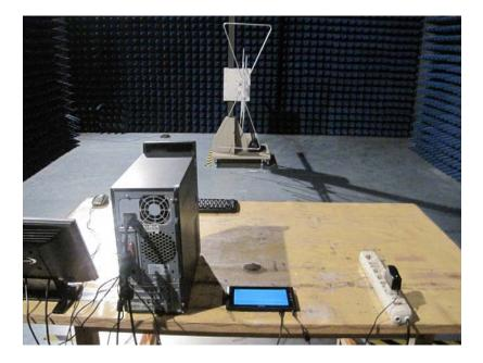
2.4 Photograph – Radiation Spurious Emission Test Setup for CTX/CRX mode Below 1GHz
