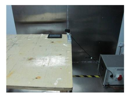
2.3 Photograph – Radiation Emission Test Setup for Communication with PC
