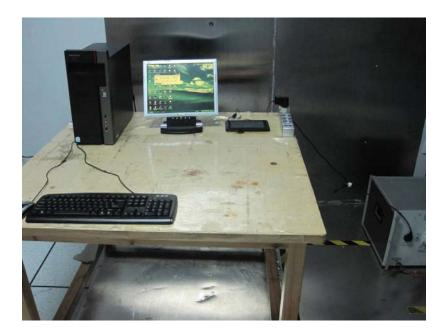
2.2 Photograph – Conducted Emission Test Setup for Normal Link mode
