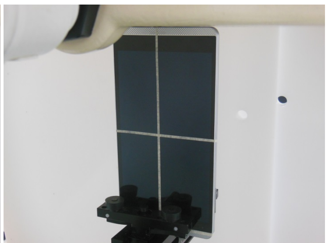
Bottom Side of the DUT with Phantom 0 cm Gap (Extremity SAR)
