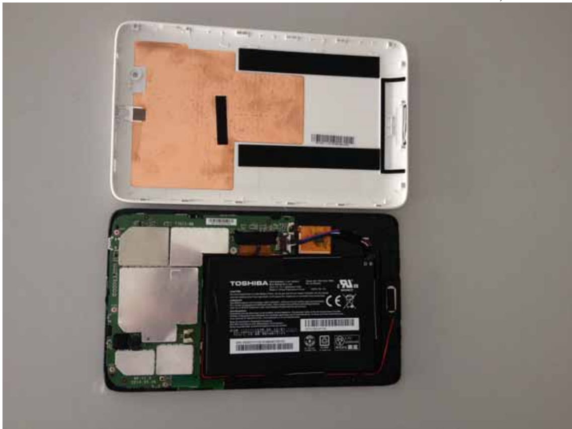
Figure 6 With Rear Camera, Inside of the EUT
