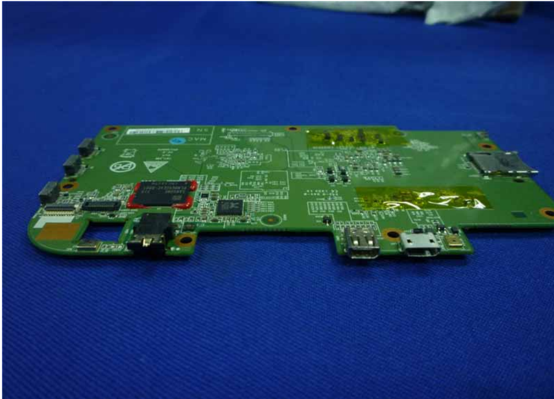
Figure 15 I/O Port of the PCB
