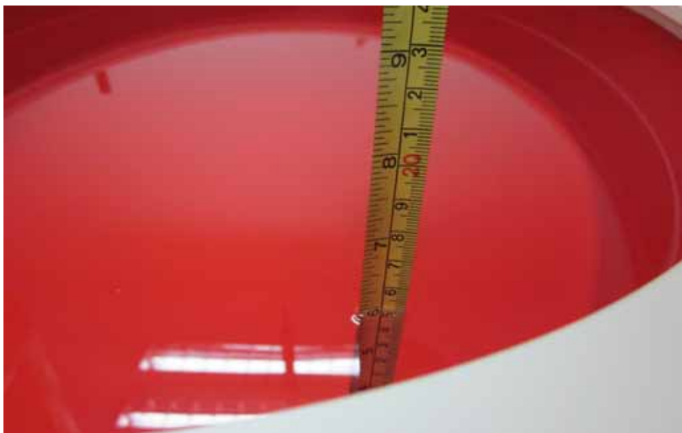
Figure 4.4: Liquid depth in the Flat Phantom
